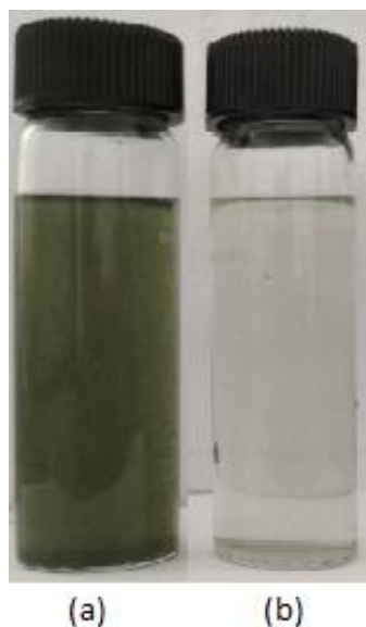
Figure 5.4: Physical appearance of TDI effluent (a) before and (b) after 60 min treatment using HC combined with Fenton's reagent
