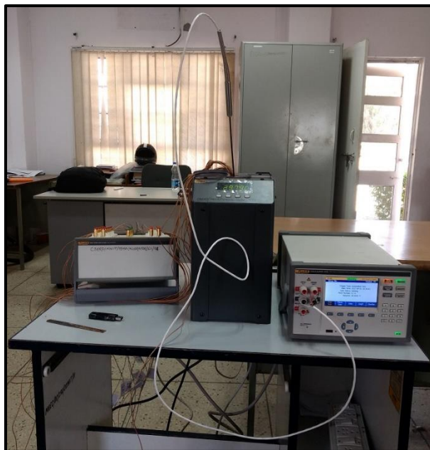
Figure 4.6: Calibration of the temperature sensors using Fluke 1586A Super-DAQ Precision Temperature Scanner
