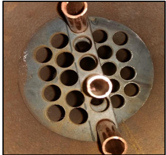
Figure 3.11: Inserting the baffle plates in the shell
