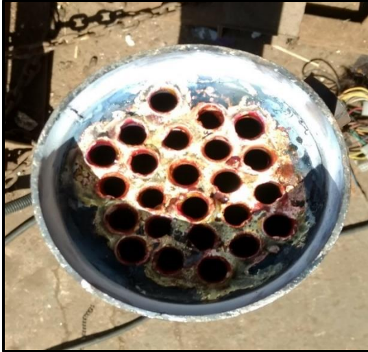
Figure 3.17: After gas tungsten arc welding of the Copper ( Cu ) tubes
