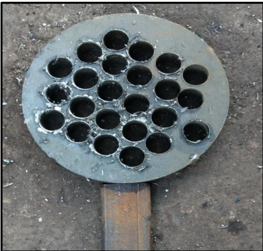
Figure 3.6: Plates after drilling
