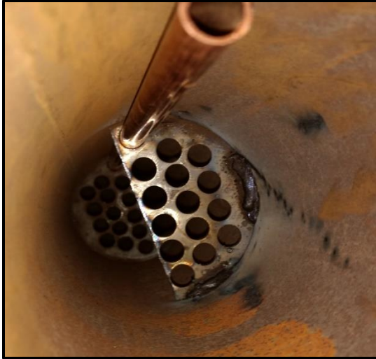
Figure 3.13: After welding of both the baffle plates
