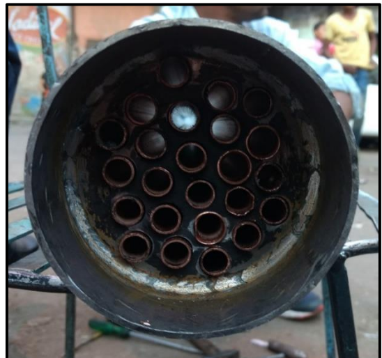
Figure 3.16: After insertion of the Copper (Cu) Tubes
