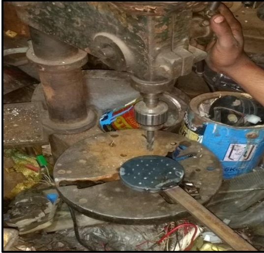
Figure 3.5: Drilling of the plates
