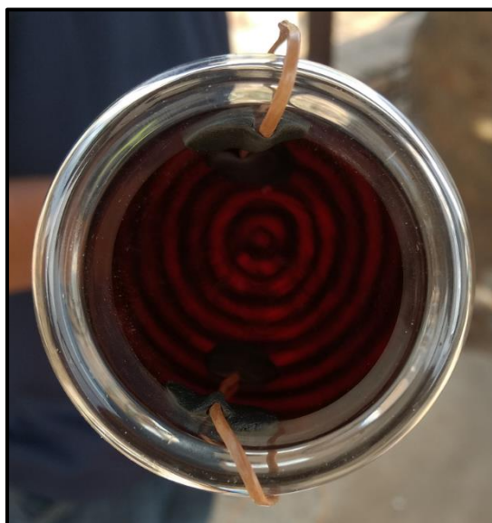
Figure 4.3: An evacuated tube with inlet and outlet temperature sensors
