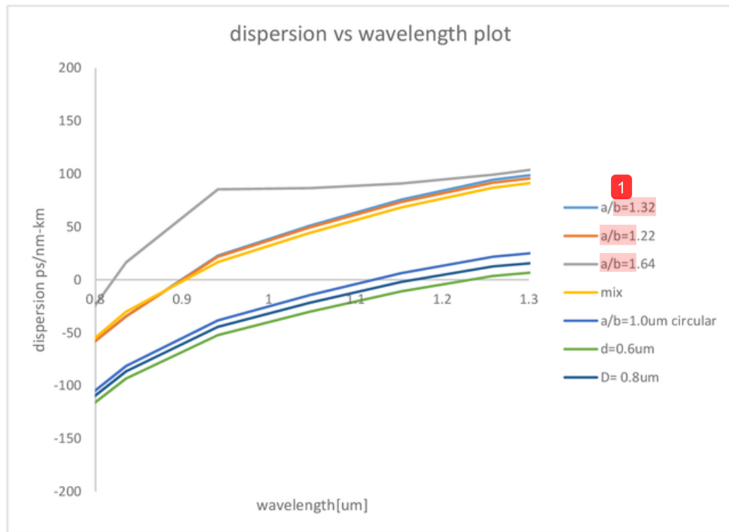
Fig 5.4(a) zero dispersion wavelength at diameter = 1 μm, 0.8 μm, 0.6 μm
