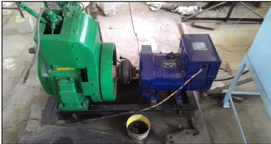
Figure 3.1: Kirloskar Diesel Engine coupled with Electrical Dynamometer
