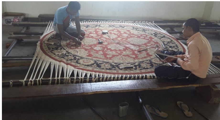
Figure 27 Removing the defects in carpets alignment
