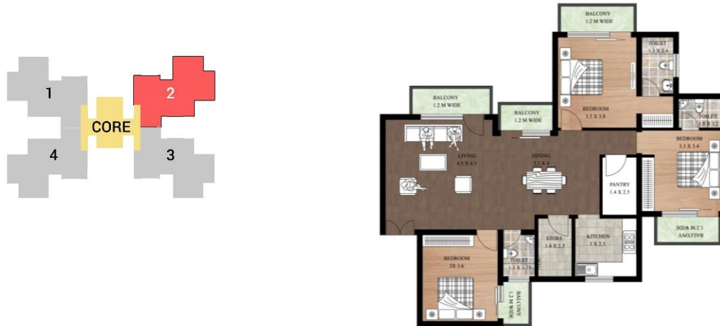
Figure 3.36 Detail of cluster and unit plan of the HSIIDC Apartments, Sector 31, Gurugram
