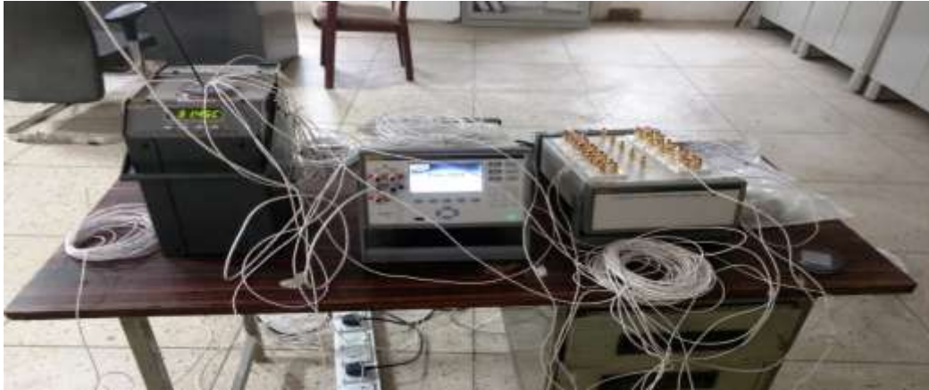
Figure 6-7: Calibration of RTD sensors using Fluke thermal calibrator
