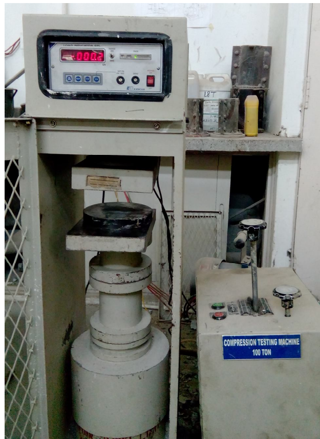
Figure 4.2: The compression testing machine for the testing of geopolymer mortar
