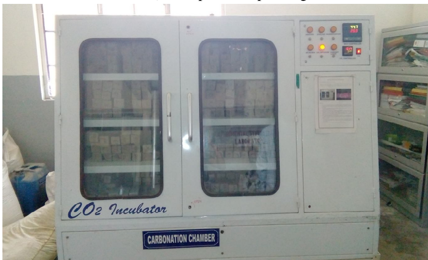
c) Samples within the carbonation chamber
