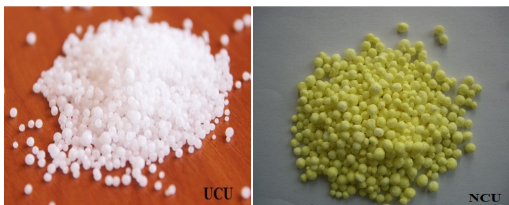
Figure 3.1. (b) NCU obtained from UCU after coating in Fluidized bed coater
