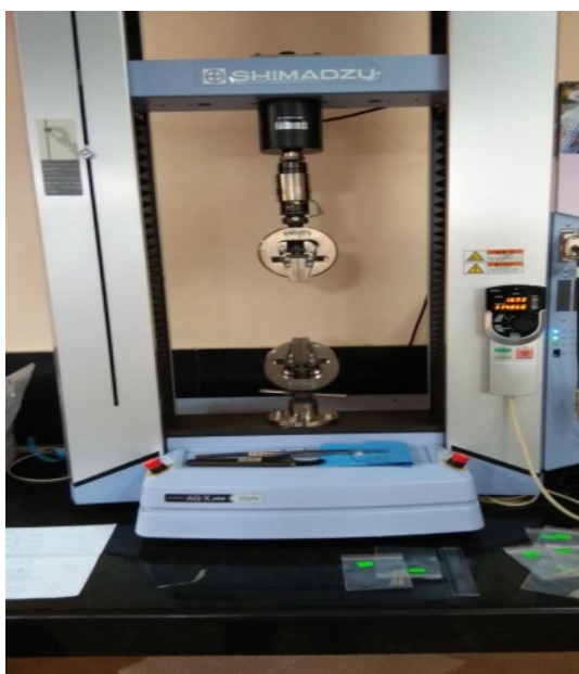
Figure 3.3. Tensile strength tester used for UCU and NCU particle
