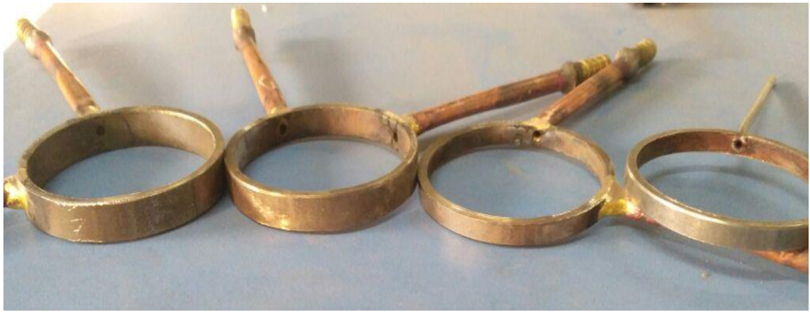
Figure 4.3 : Argon Gap Rings of Different Thicknesses with Permeate Collector and Gas Supply Connector
