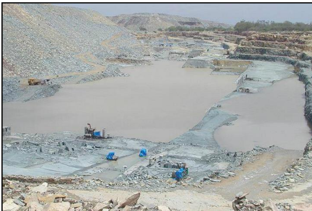
Figure 1.6: Exhaustive Kota stone Mining site and in the Background, Piles of Waste Generated During the Mining Process.
