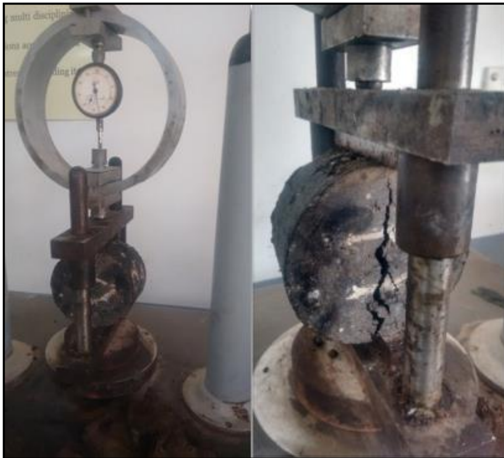
Figure 3.6: Laboratory Test Setup for the Indirect Tensile Strength Test.
