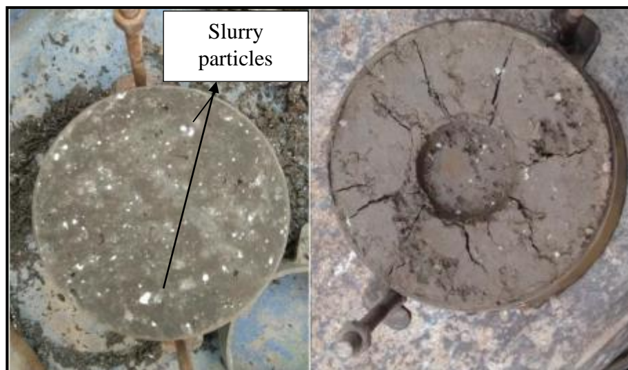
Figure 3.2 CBR Sample Before and After Testing
