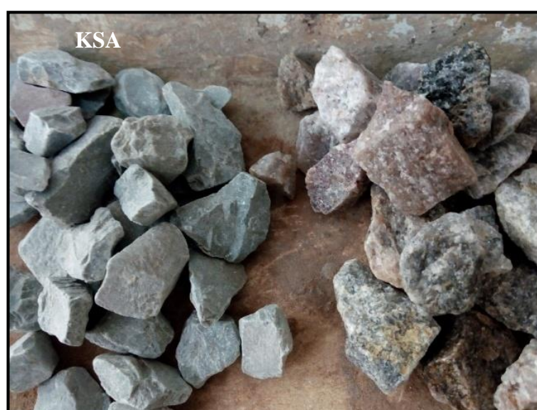
Figure 4.13: Texture Difference of Kota Stone Aggregates (left) Compared to Conventional Aggregate (right)
