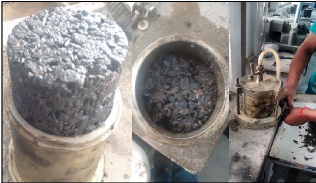
Figure 3.13: Falling Head Permeability Test Setup for OGFC.
