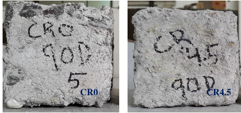
Fig. 6.15: Acid attacked crumb rubber concrete samples
