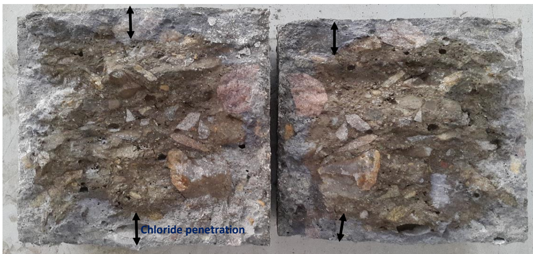
Fig. 6.9: Chloride penetration in crumb rubber concrete specimens
