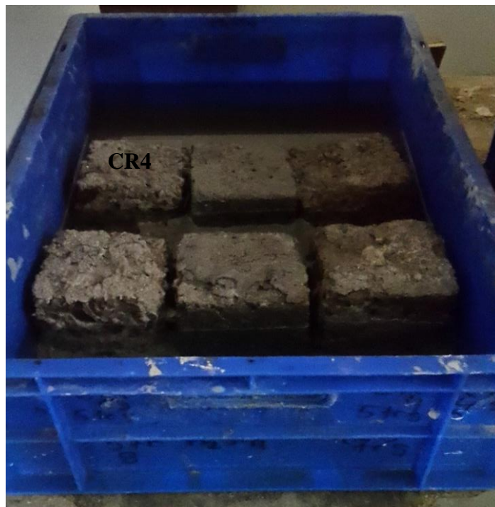
Fig. 6.6: Specimens exposed to acidic environment
