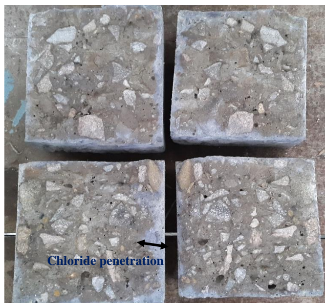
Fig. 6.25: Depth of chloride penetration in waste glass concrete specimens
