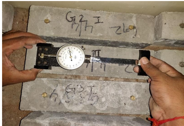
Fig. 5.3: Drying shrinkage of specimens
