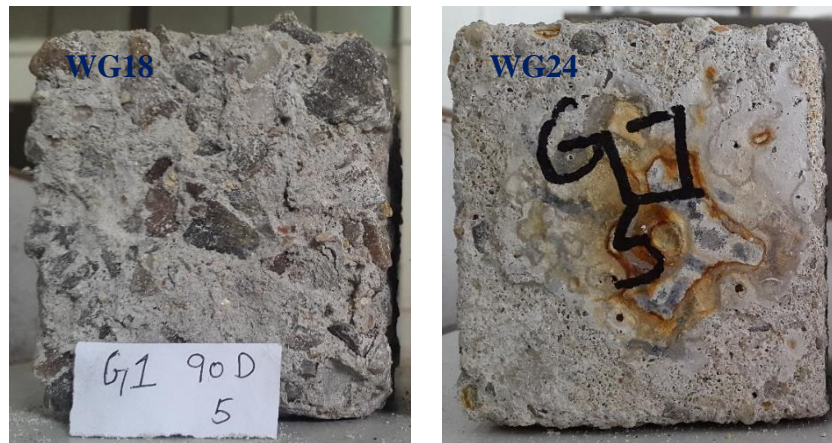
Fig. 6.31: Acid attacked waste glass concrete samples
