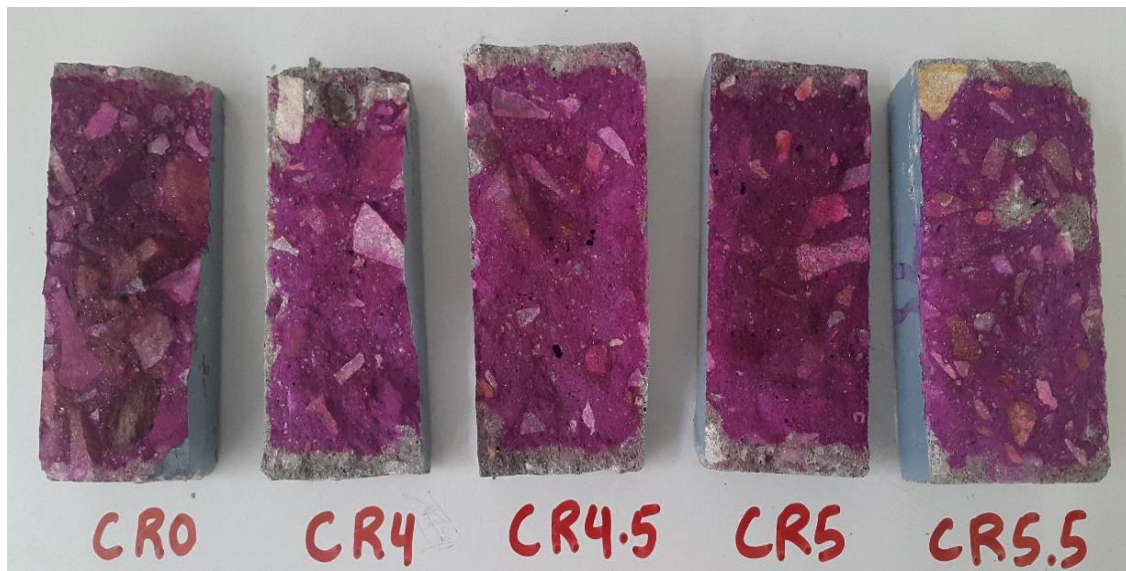
Fig. 6.12: Carbonation depth of crumb rubber concrete prisms after exposure to 28 days
