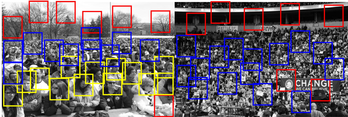
Figure 3.14: Experimental results of head detection: left side image of our dataset provides little bit of considerable outcomes of head detection. The red boxes represent false positives, blue represents false negative, while the yellow one represents correct detections. However, both images are evidence of false negatives and false positives.
