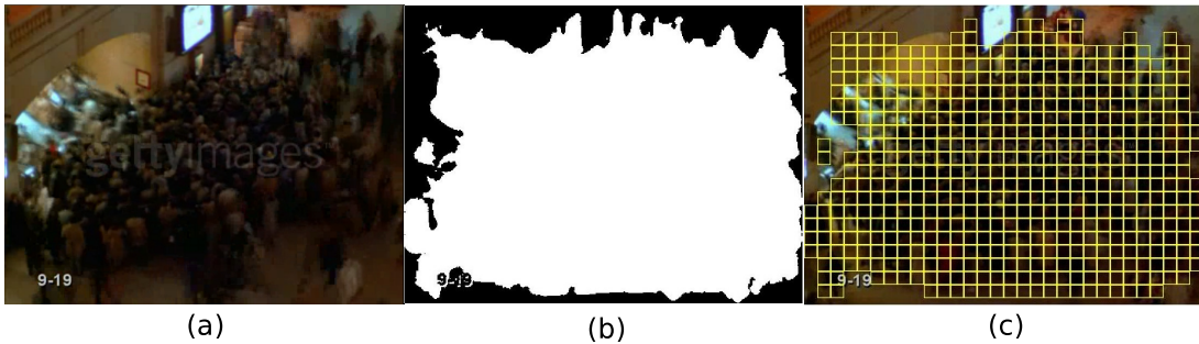
Figure 4.2: (a) Sample video frame (b) segmented foreground region using active contour approach (c) the segmented region is further divided into blocks.
