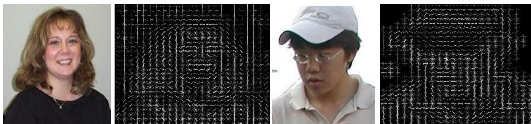
Figure 3.6: An example: HOG feature visualization of training images used in face detection.
