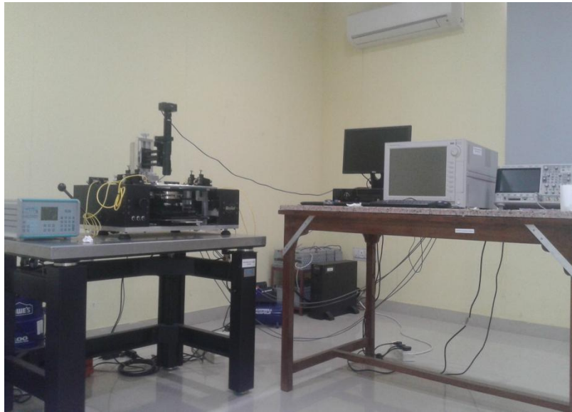
Figure 3.16: Semiconductor Device Analyzer (Agilent B1500A) with probe station at MRC, MNIT Jaipur.
