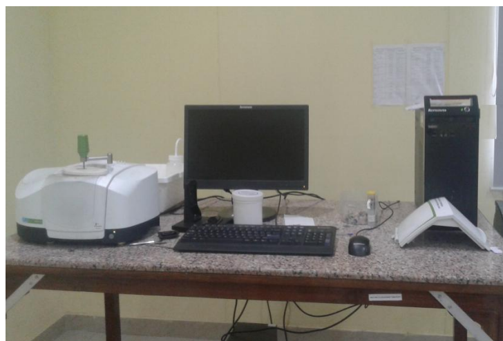
Figure 3.14: Fourier Transform Infrared Spectroscopy (FT-IR Spectrum 2 Perkin Elmer) at MRC, MNIT Jaipur.
