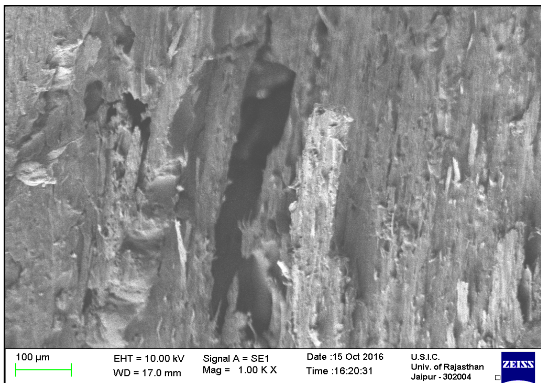
Figure 4.30 [a]: Nylon 66+2wt. % TiO 2 (Load: 100 N, Sliding Velocity: 6.5m/s, Sliding Distance: 2000m)
