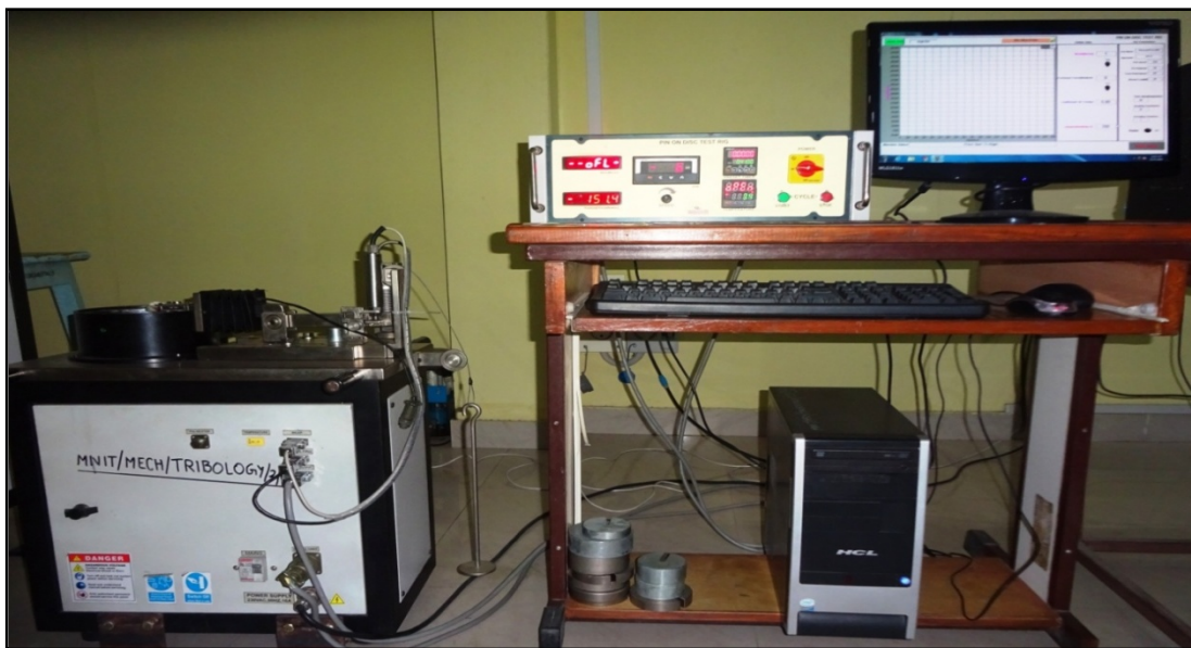
Figure 3.13: Pin-on-disc type wear and friction monitoring test rig
