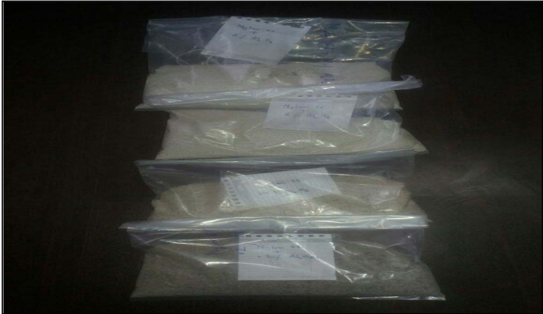
Figure 3.3: Polymer composite granules of Nylon66 and \text{Al}_2\text{O}_3
