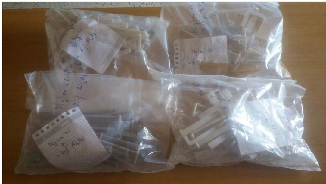
Figure 3.7: Test specimens prepared by Injection Moulding
