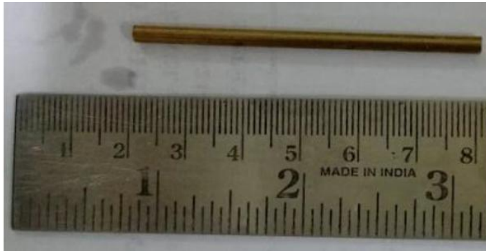
Figure C.1 Initial brass tool electrode ( \Phi= 3 )
