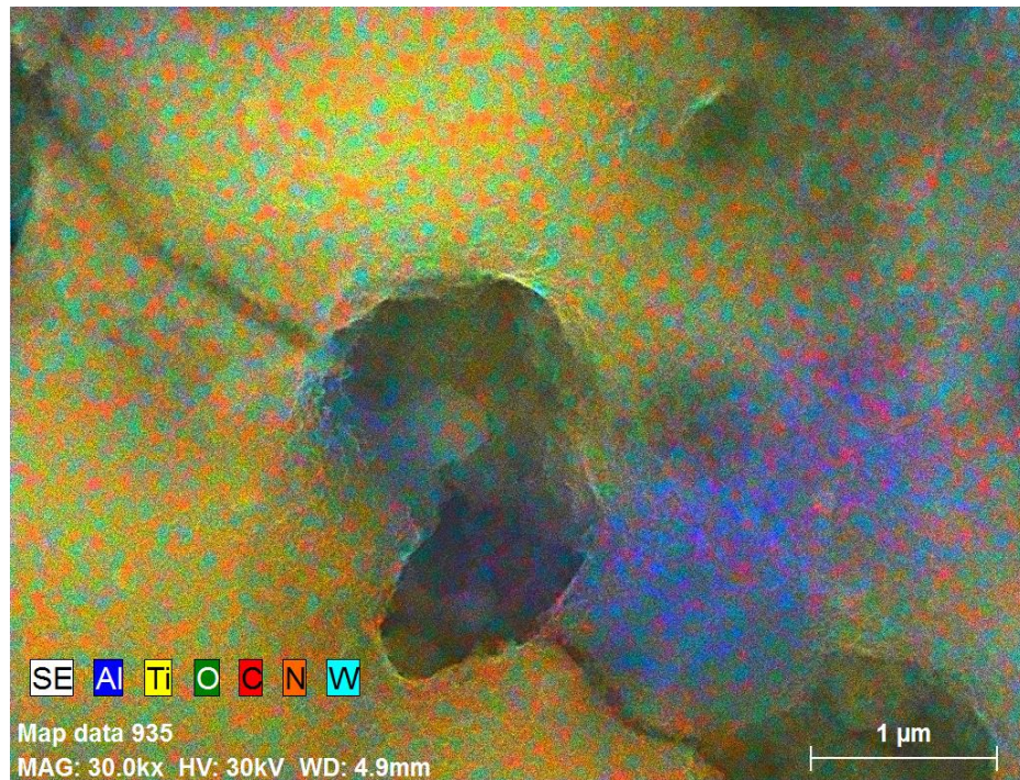
Figure 5.18 SEM image of ED milling surface for EDS
