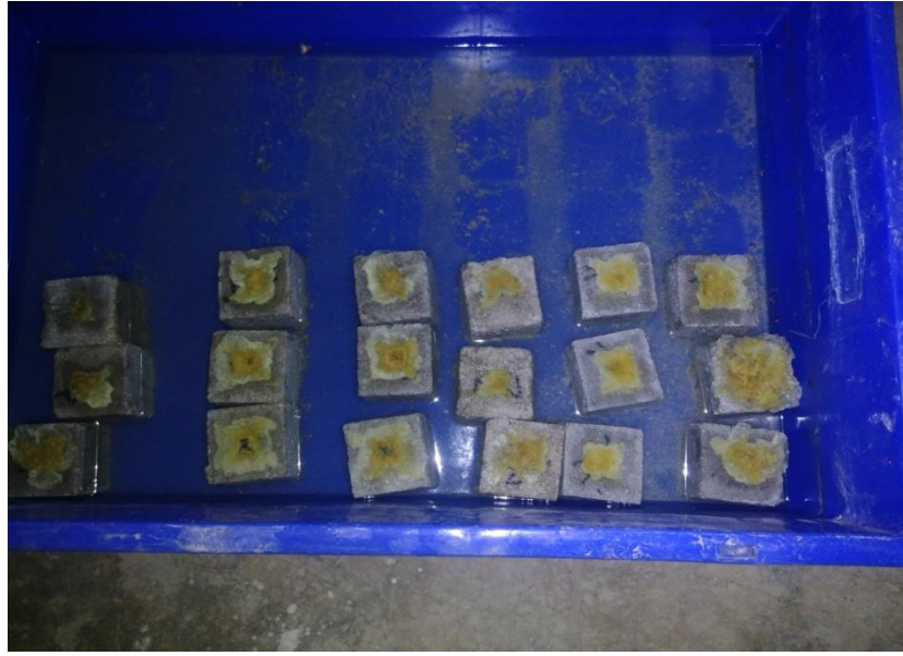
Figure 1.5 Cube in H_2SO_4 solution
