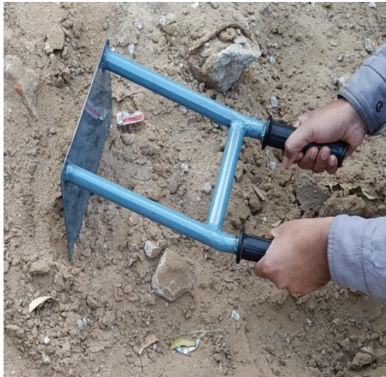
Figure 5.13: Newly designed clot cutting/mud pulling hand tool
