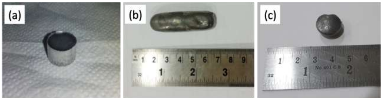
Fig. 3.1 (a) cold compacted pellet and as casted HEA samples in (b) cylindrical shape and (c) button shape
