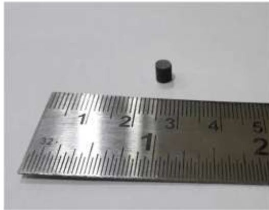
Fig. 3.2 Specimen for compression test
