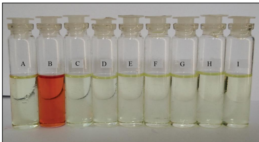
Fig. 1 – Colour changes in the receptor RC ( 1 \times 10^{-5} M in DMSO) in presence of 10 equivalents of different anions (as their TBA salts). [A, B, C, D, E, F, G, H and I represent receptor RC , RC +F - , RC +Cl - , RC +Br - , RC +I - , RC +CH 3 COO - , RC +H 2 PO 4 - , RC +HSO 4 - and RC +NO 3 - respectively].
