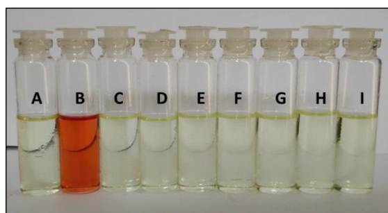
Fig. 4.6: Colour changes in the receptor RC ( 1 \times 10^{-5} M in DMSO) in presence of 10 equivalents of different anions (TBA salts) where A, B, C, D, E, F, G, H and I represent receptor RC , RC + \text{F}^- , RC + \text{Cl}^- , RC + \text{Br}^- , RC + \text{I}^- , RC + \text{CH}_3\text{COO}^- , RC + \text{H}_2\text{PO}_4^- , RC + \text{HSO}_4^- and RC + \text{NO}_3^- ions respectively
