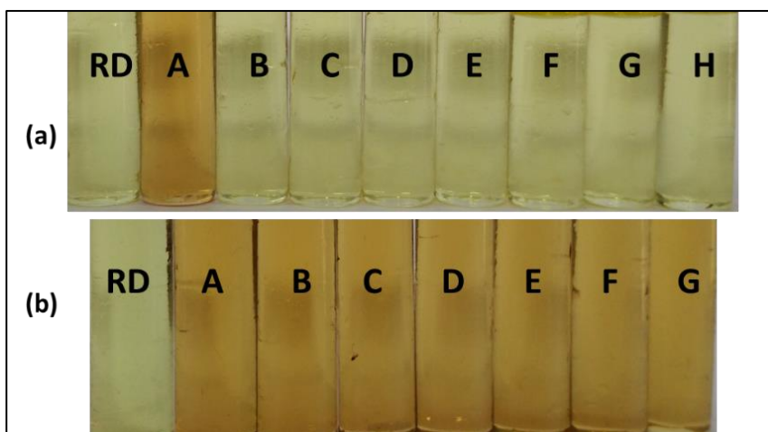
Fig. 5.6: (a) Colour changes in the receptor RD ( 1 \times 10^{-4} M in DMSO), in presence of 1equivalent of different anions (TBA salts) in 9:1 DMSO-water, where A, B, C, D, E, F, G and H represent F^- , Cl^- , Br^- , I^- , CH_3COO^- , H_2PO_4^- , HSO_4^- and NO_3^- ions, respectively. (b) Colour changes in the receptor RD ( 1 \times 10^{-4} M in DMSO), in presence of 1equivalent each of fluoride and different anions (TBA salts) in 9:1 DMSO-water, where A, B, C, D, E, F, G and H are receptor and, F^- + Cl^- , F^- + Br^- , F^- + I^- , F^- + CH_3COO^- , F^- + H_2PO_4^- , F^- + HSO_4^- and F^- + NO_3^- , respectively
