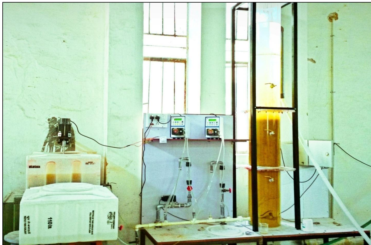
Figure 3.4: Fully functional Pilot plant with established sludge blanket
