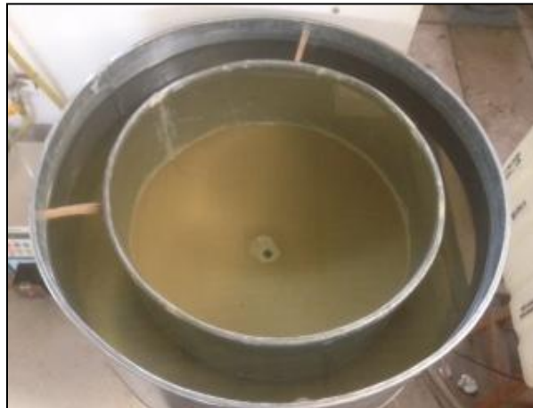
Figure 3.6: Flocculator and Clarifier of Conventional clariflocculator model
