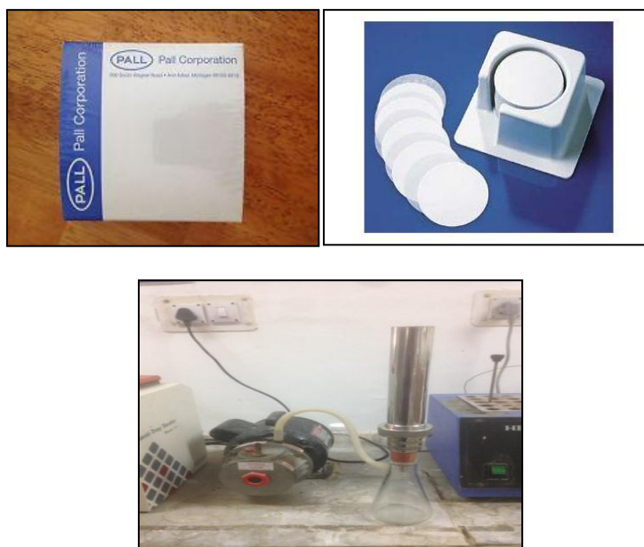
Figure 3.17: Dissolved Al measurement with 0.45 \mu filter paper and vacuum filter
