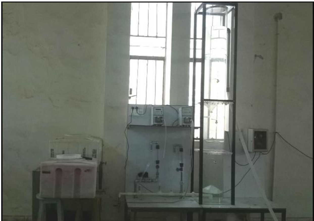
Figure 3.2: The Pilot plant of Pulsator installed at Hydraulics lab, MNIT Jaipur .
