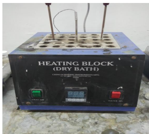
Figure 6: Closed reflux apparatus
