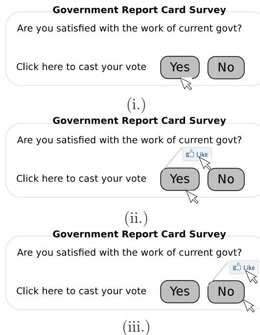
FIGURE 6.3: Workflow for our advanced transparency attack using SVG filters. At first, (i) displays the normal working when user clicks “Yes” button, (ii) When the user clicks on Yes button a Facebook “like” button is clicked, (iii) When the user clicks on “No” button, still Facebook “like” button is clicked.
