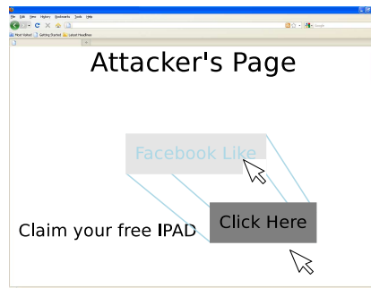
FIGURE 6.1: Illustration of clickjacking attack using frame overlays. In this attack, a Facebook page is embed on a transparent iframe. Facebook “ like ” button is shown with light colour in a figure to represent invisibility.
