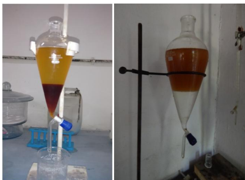
Fig. 3.1 (a) Transesterification set up (b) Methyl alcohol and Potassium hydroxide (c) Biodiesel and glycerol layers (d) Water washing of biodiesel
