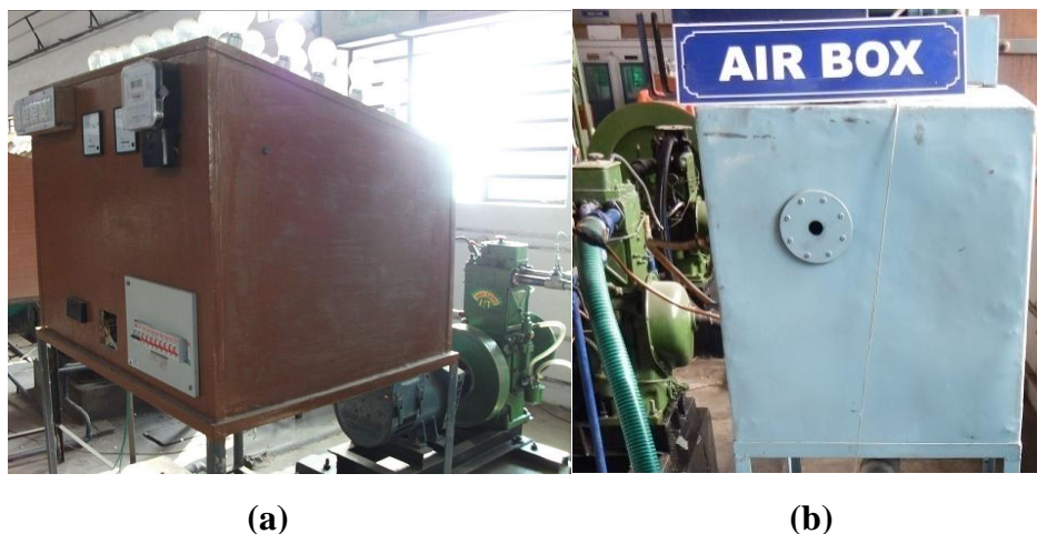
Fig. 4.5 (a) Electrical load bank (b) Air box with orifice
