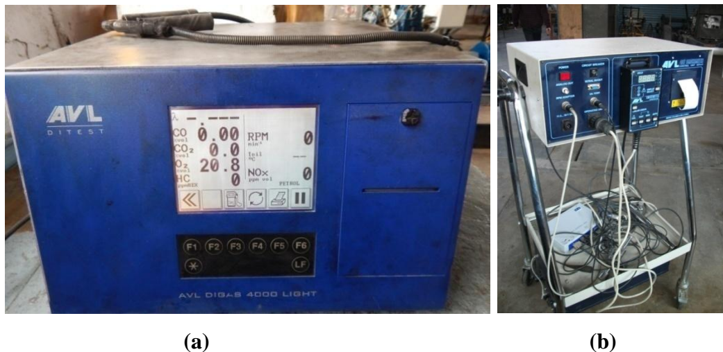
Fig. 4.9 Exhaust gas composition measurements (a) five-gas analyser (b) Smoke meter
