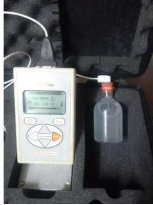
Figure 20 KD-2 pro for thermal conductivity measurement
