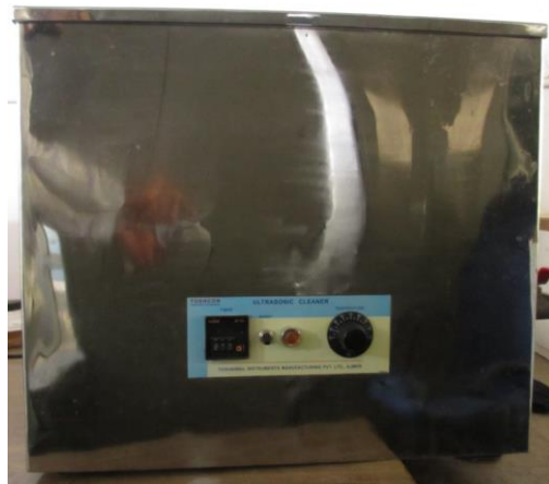
Figure 19 Ultrasonic cleaner with 45 litre capacity
