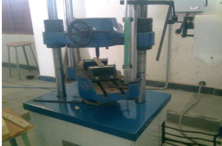
Fig.18 Flexural test on Universal Testing Machine
