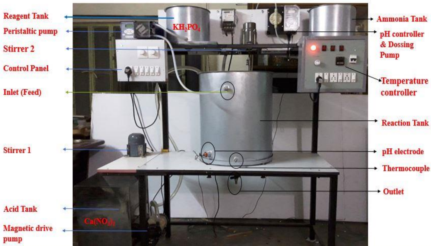
Figure 5-7. Pilot scale lab reactor for synthesis of MA-Hap LR
