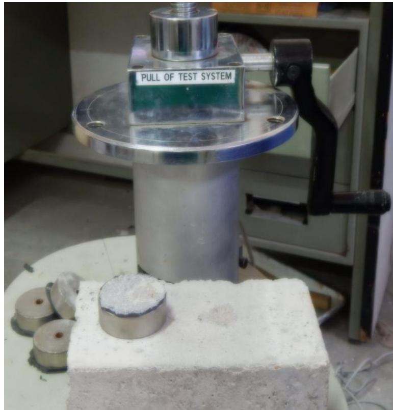
Figure 3.17: Pull-off Strength test apparatus
