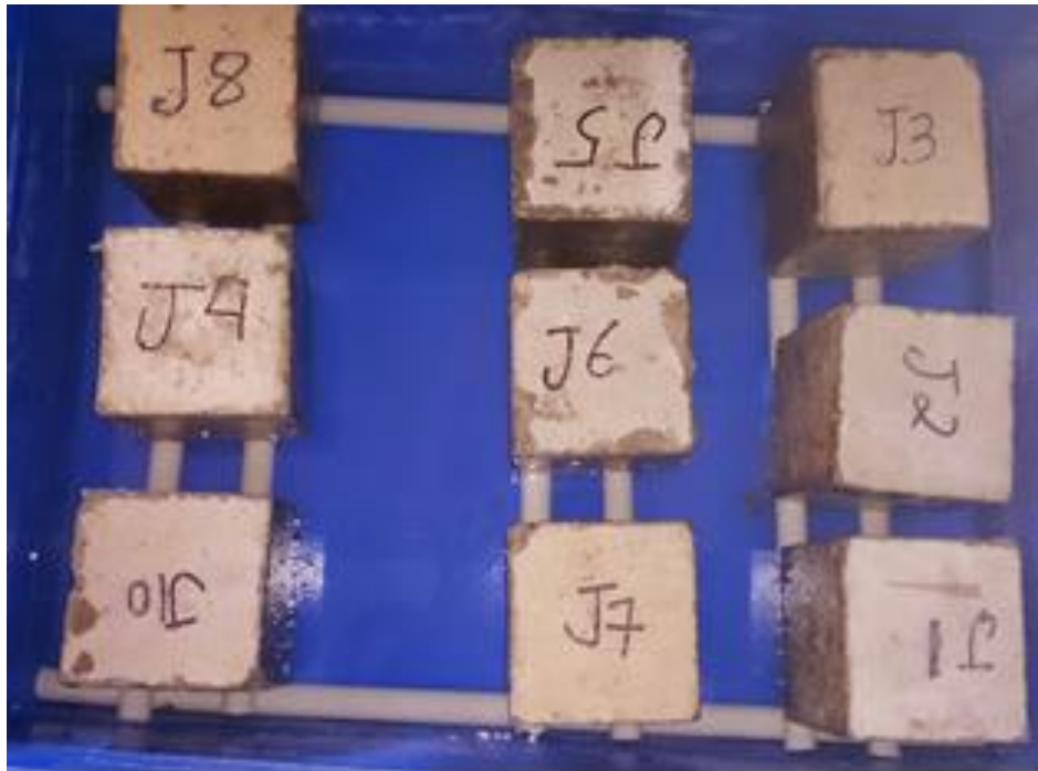
Figure 3.8 Concrete Samples (Series I) Placed on Rods for Capillary Action
