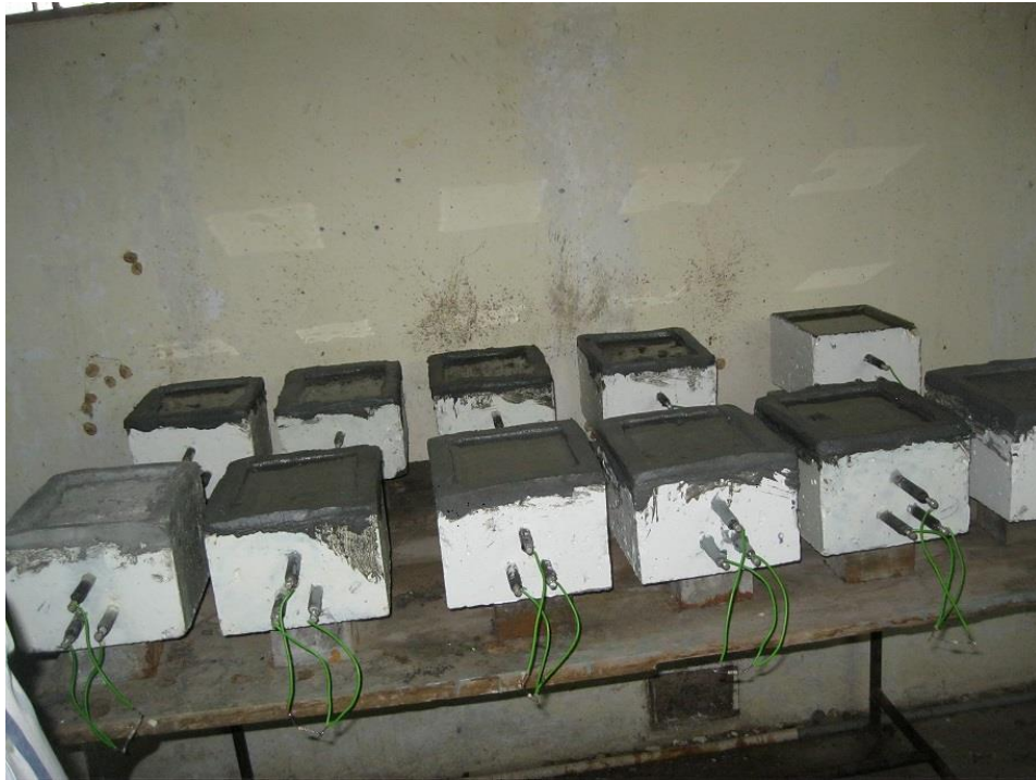
Figure 4.19 Connections of Bars for Half Cell Potential
