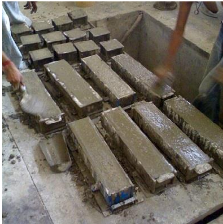
Figure 3.7 Casting of 100 \times 100 \times 100 mm Cubes and 100 \times 100 \times 500 mm Beams.
