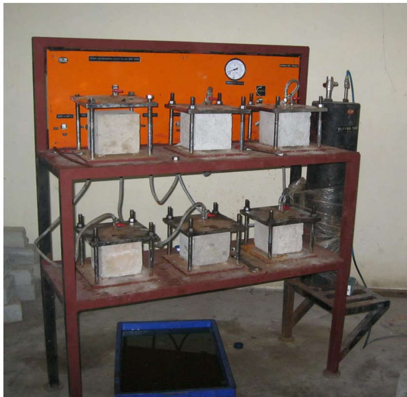
Figure 3.11 DIN 1048 Apparatus for permeability test
