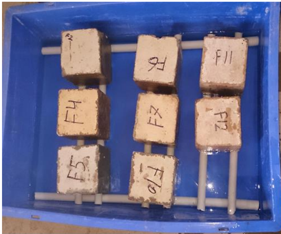
Figure 3.9 Concrete Samples (Series II) Placed On Rods for Capillary Action
