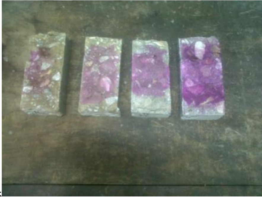
Figure 4.14 Samples Showing Carbonated Depth of Sliced Samples for Series II
