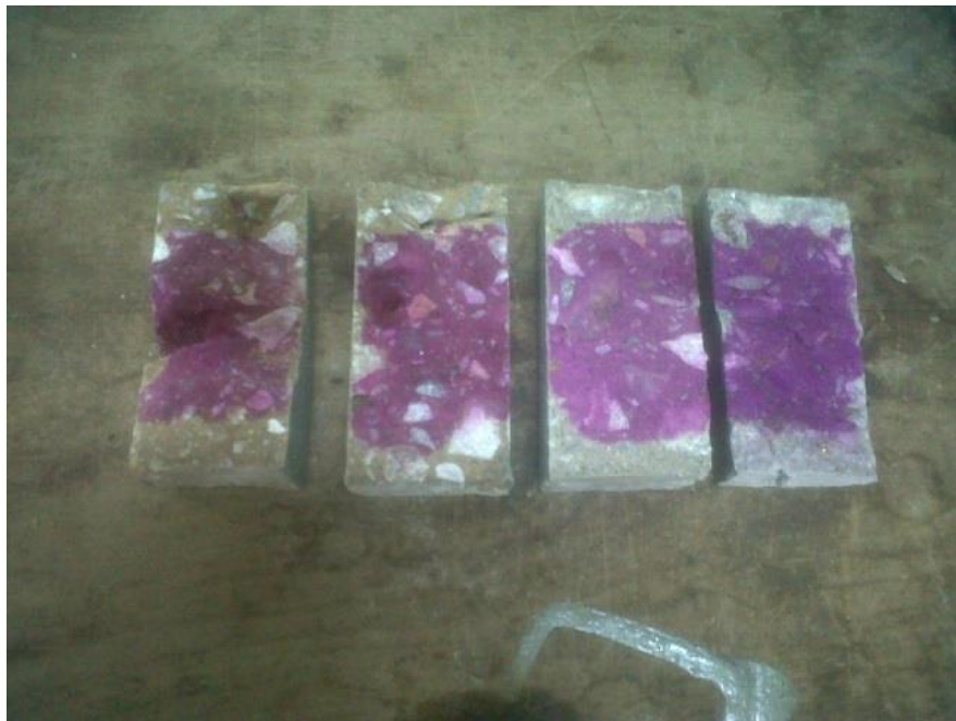
Figure 4.13 Samples Showing Carbonated Depth of Sliced Samples for Series I
