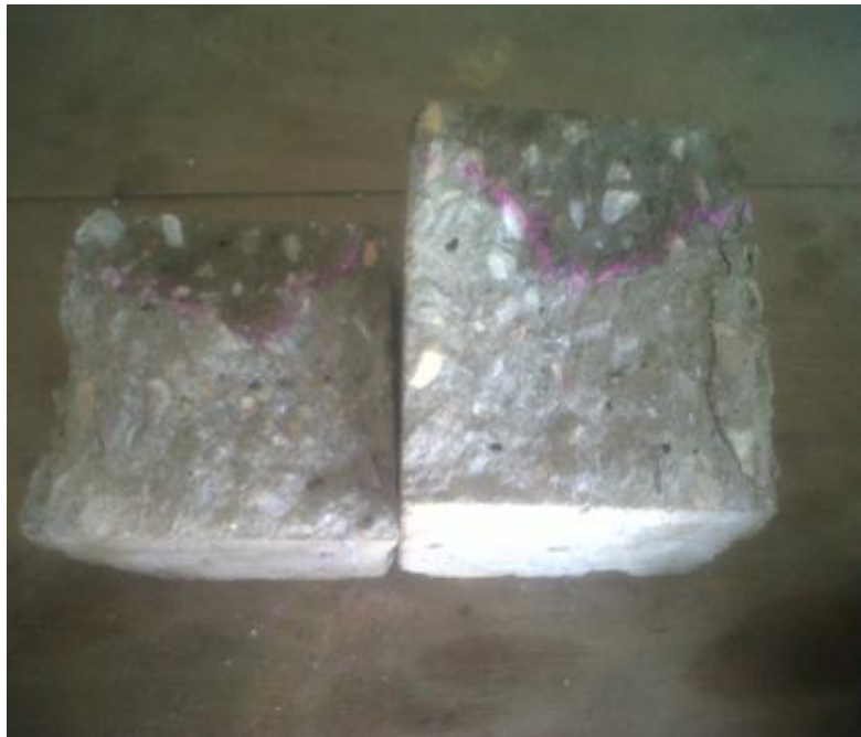
Figure 4.7 Concrete Samples (Series II) Showing Penetration of Water
