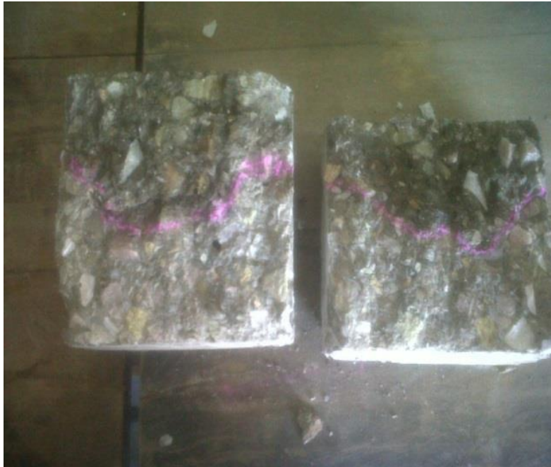
Figure 4.6 Concrete Samples (Series I) Showing Penetration of Water
