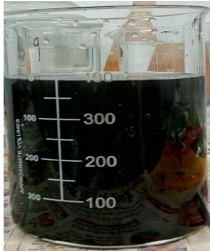
Figure 3.2 Sample of homogeneous EG/water suspension just after preparation
