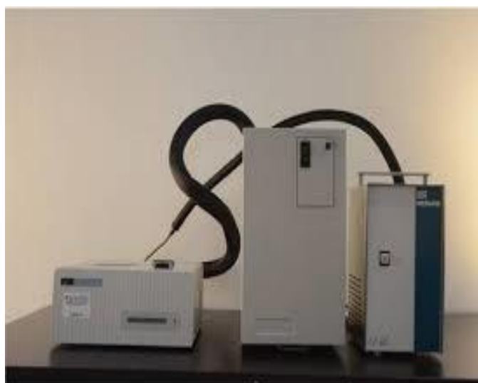
Figure 3.7 Pris 6 DSC instrument
