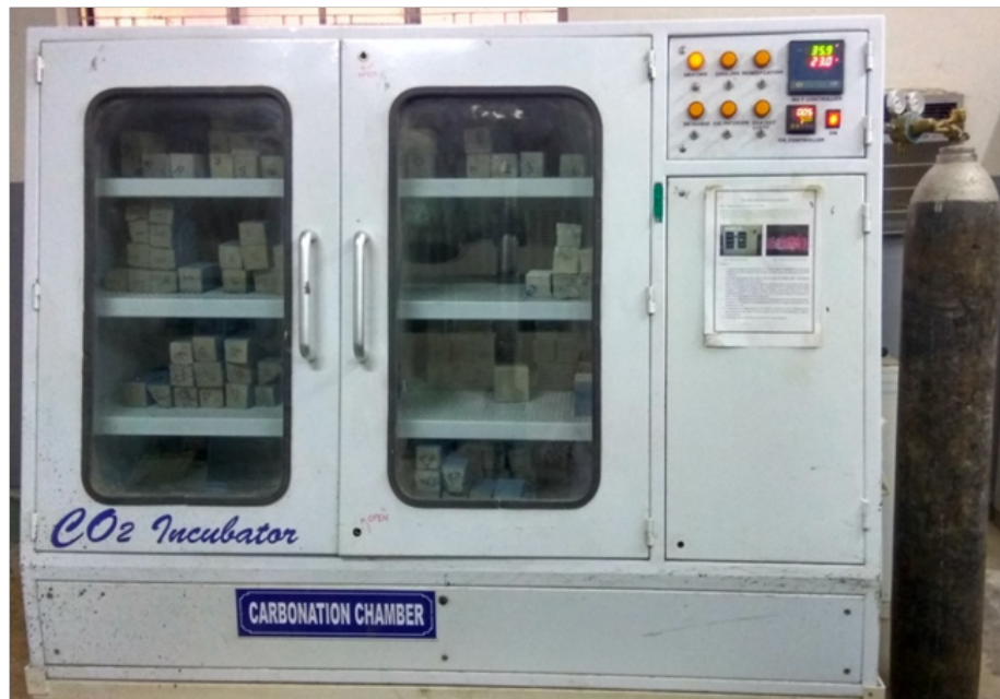
Figure 2.18: Carbonation chamber setup
