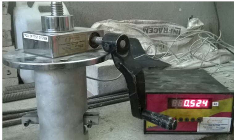
Figure 2.16: Pull-off test setup
