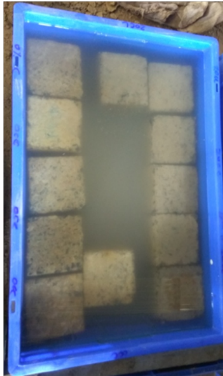
Figure 2.20: Specimen immersed in sulfate solution
