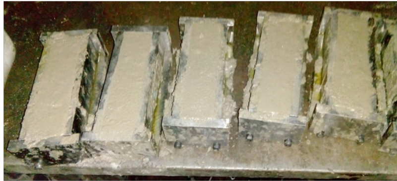
Figure 5.25: Casting of carbonation moulds
