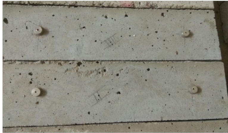
Figure 2.19: Shrinkage specimen with studs
