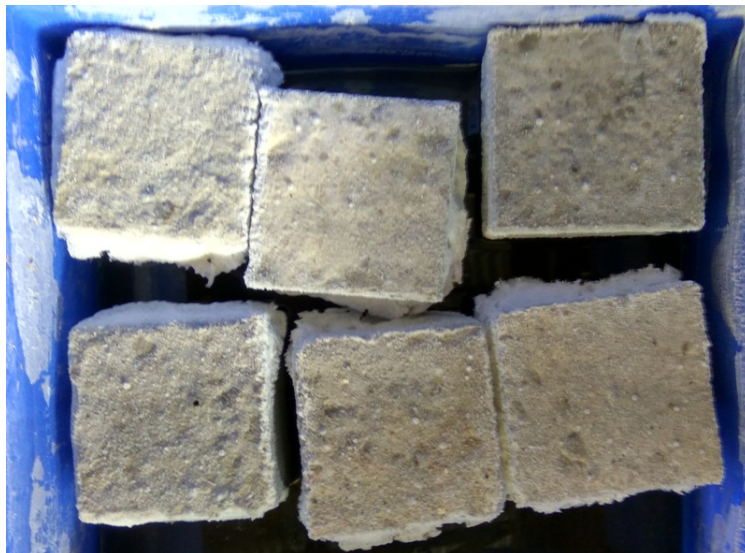
Figure 3.13: Physical appearance of geopolymer and OPC concrete
