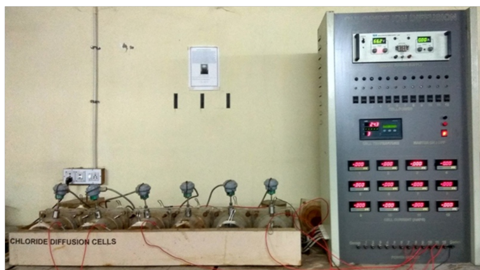
Figure 2.25: Chloride migration setup
