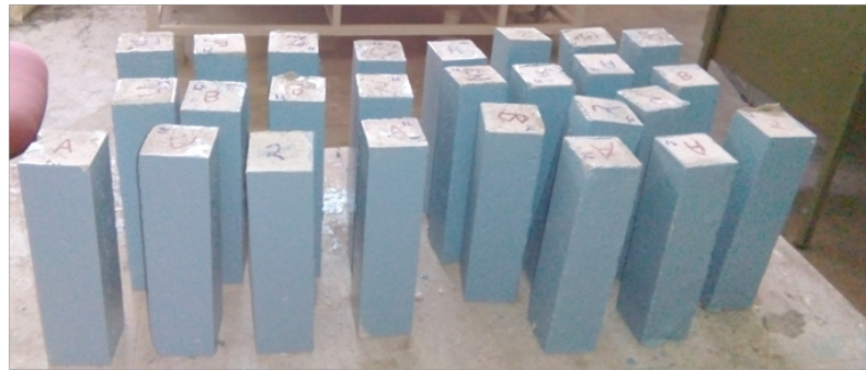
Figure 5.26: Preparation of carbonation moulds
