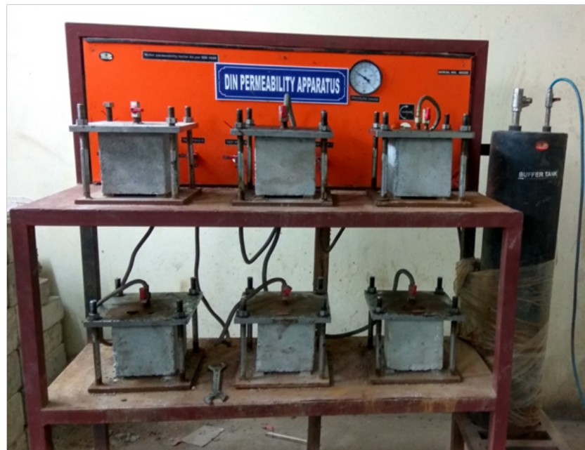
Figure 2.17: DIN 1048 water permeability test setup
