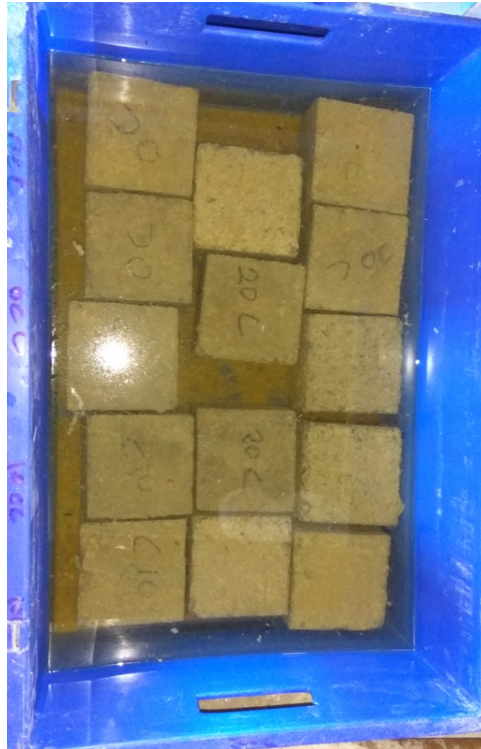
Figure 2.22: Specimens immersed in salt solution
