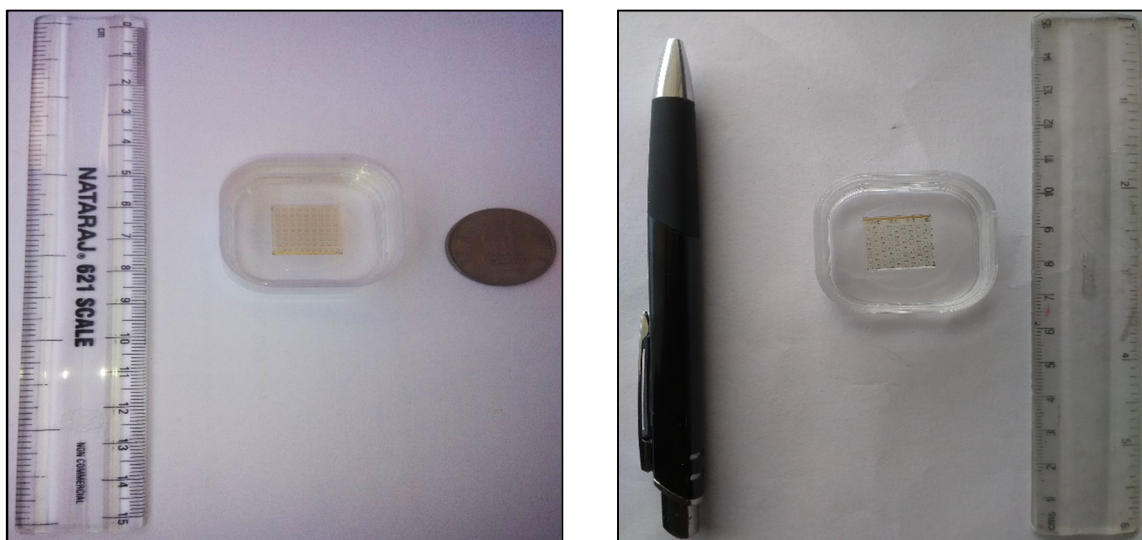
Figure 7.11: Snapshot of the prepared PhC LTS based superlattice InGaN/GaN solar cell; (a) in comparison with a coin, (b) in comparison with a pen.
