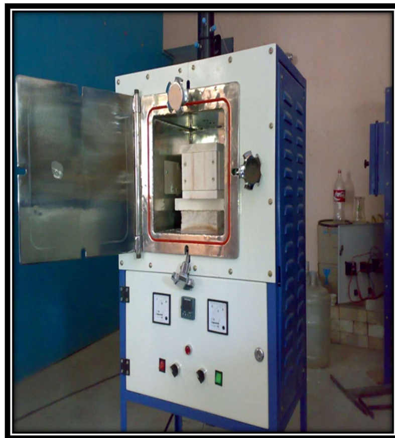
Figure 3.5: Microwave sintering furnace with its ceramic cavity
