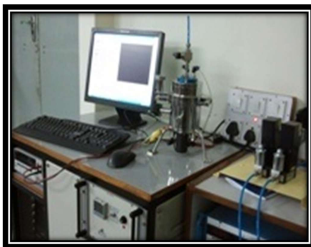
Figure 3.22: Image of custom-built setup using Keithley- 2400 SMU
