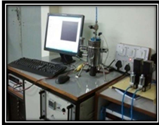
Figure 3.14: Custom built I-V measurement and gas sensing set up
