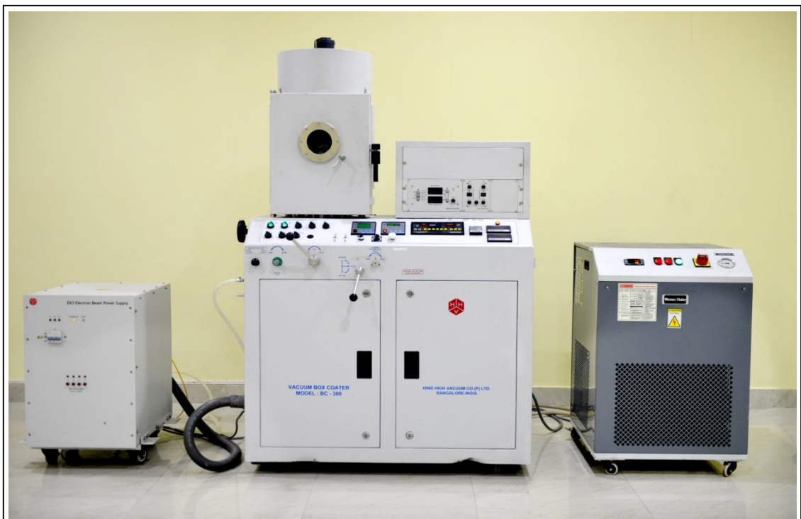
Fig.3.4 Experimental setup of thermal vapor evaporation technique (Model: BC-300 HHV).
