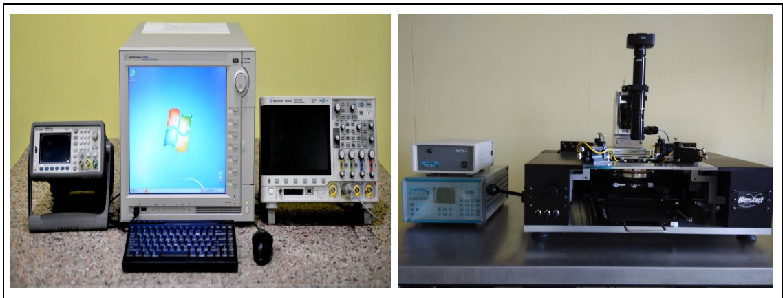
Fig.3.18 Setup for I-V/ C-V measurement (a) measuring unit (Model: Agilent-B1500A) (b) probe station.
