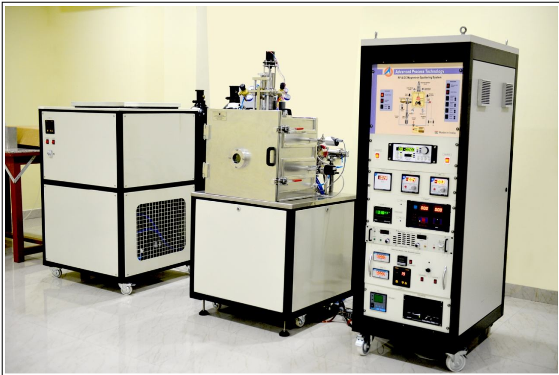
Fig.3.2 Experimental setup of RF sputtering system (Company: Advanced Process Technologies, India).
