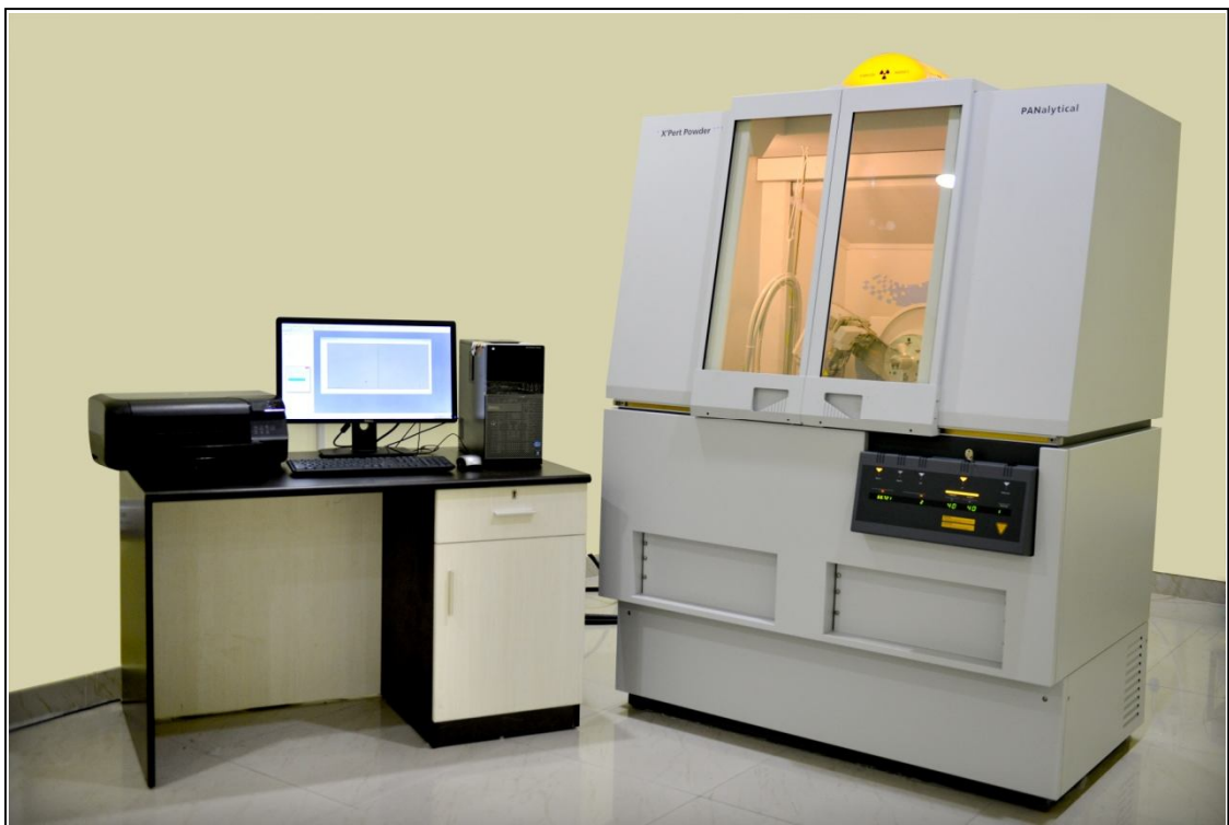
Fig. 3.6 Experimental setup of X-Ray diffraction system (Model: PANalytical X'Pert Pro).
