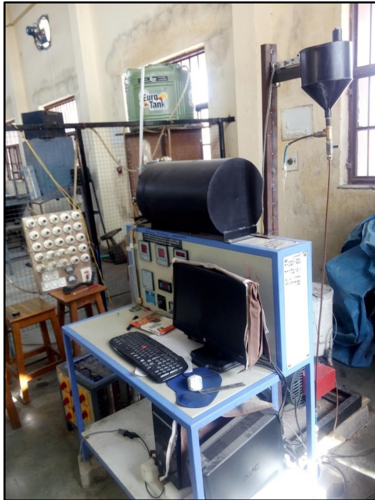
Fig 3 2. Single Cylinder Constant Speed Stationary C.I Engine
