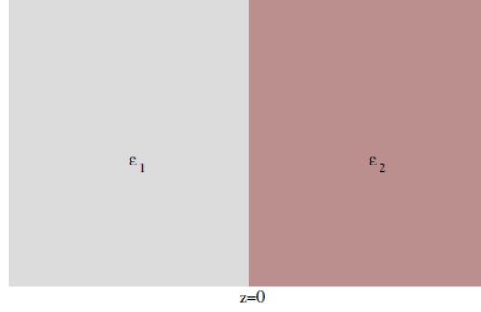
Figure 1.2: Two semi-infinite media with dielectric functions \varepsilon_1 and \varepsilon_2 separated by a planar interface at z = 0 .
