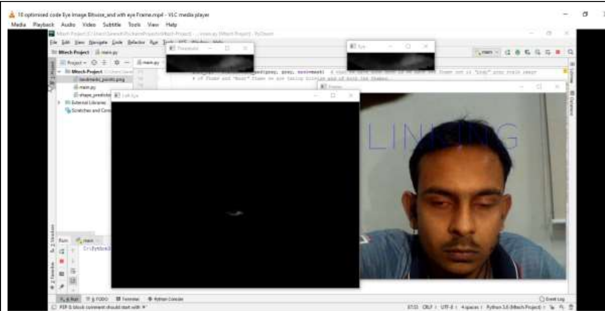
Figure 5.16 This image is output of bitwise_and structure. Here we can see blinking, which is on the main frame while the mask show us the position of the structure that is analysed to conclude blinking.
