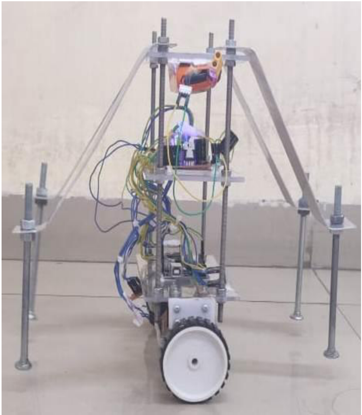
Fig. 6.9 A view of robot with four supports when it starts balancing itself
