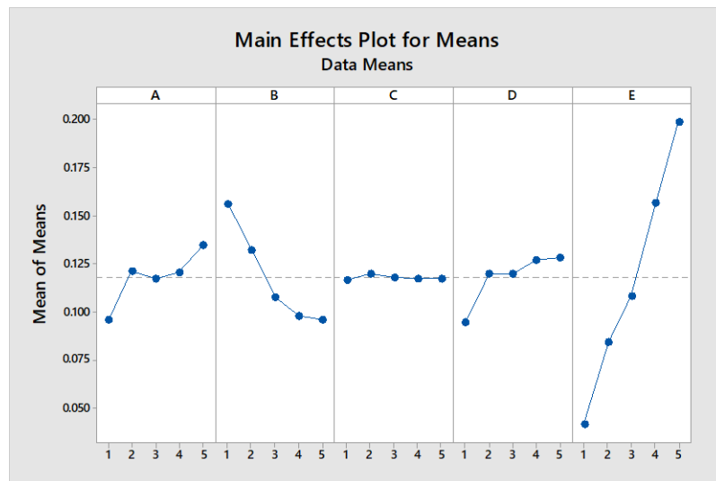
Figure 6.4. Influence of control parameters on means for AlCr 1.5 CuFeNi 2 Mn x alloys
