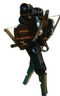
Fig. 2.24 Planar bipedal testbed MABEL (Sreenath et al., 2011)
