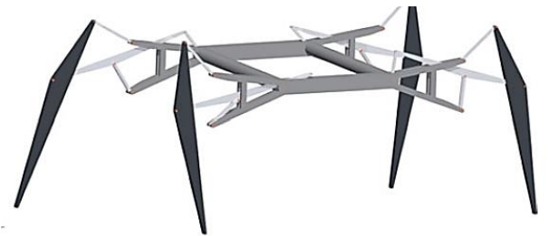
b) Stephenson III leg mechanism (Batayneh et al., 2013)
