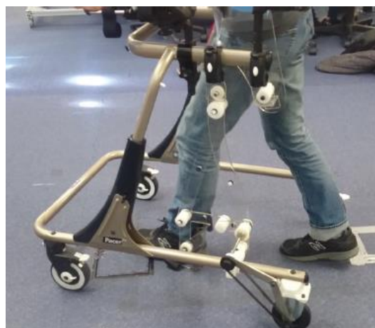
Fig. 2.9 Parallelogram mechanism at ankle joint of WalkTrainer™ (Stauffer et al., 2009)
