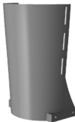
Fig. 7.5 Base model of thigh attachment used for shape synthesis of knee exoskeleton
