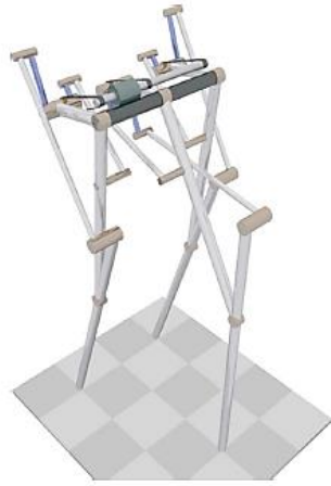
Fig 2.25 a) Single DOF planar biped (McKendry et al., 2008)
