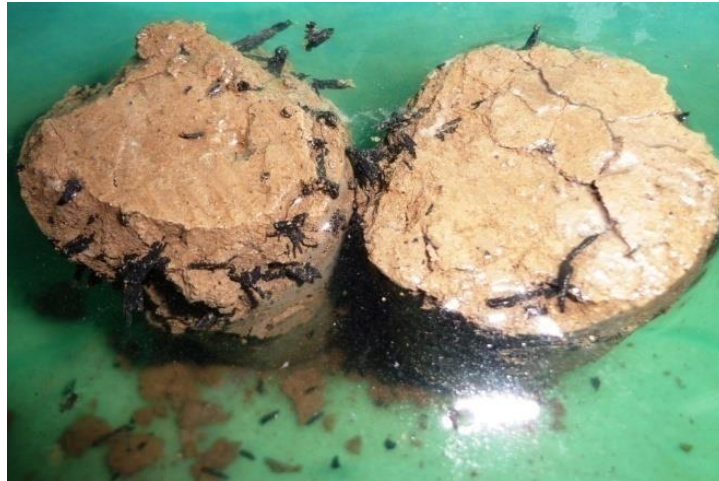
Fig. 6.9 Disintegration of specimens after being immersed in water
