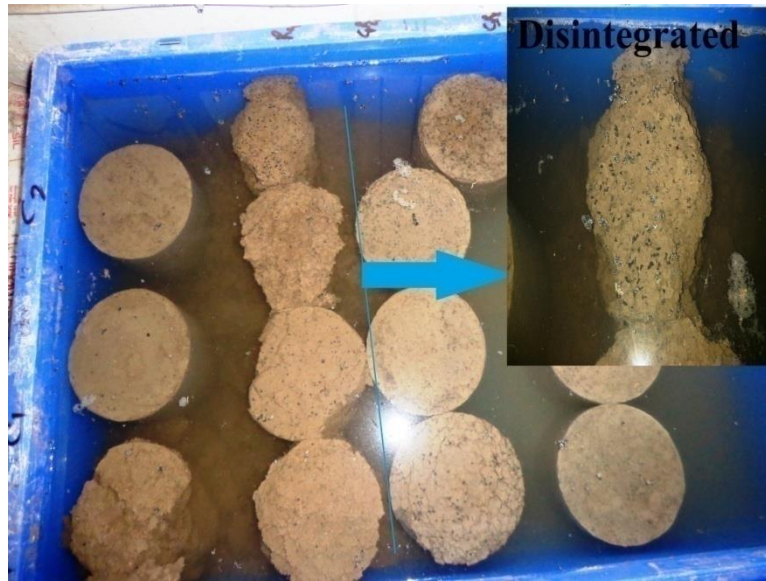
Fig. 4.36 Disintegrated specimens of clay-rubber crumbles during first cycle of durability test
