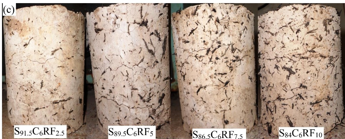
Fig. 6.50 Photographs of the clayey soil-cement-rubber fibre specimens during wetting and drying cycles (180 days cured)
