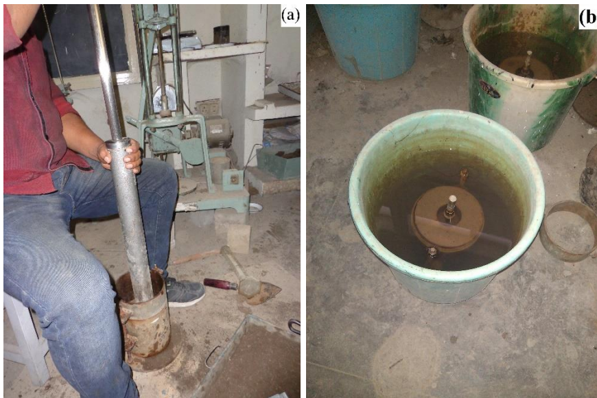
Fig. 3.10(a) Sample preparation of California bearing ratio test, (b) specimens soaked under water
