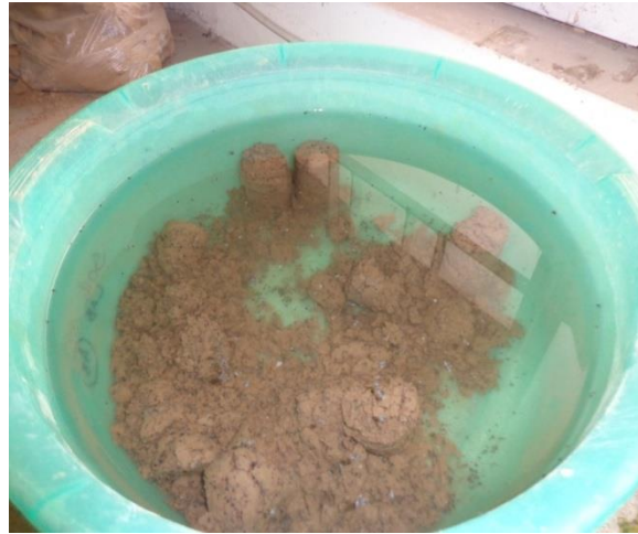
Fig. 4.15 Disintegration of clayey soil-rubber crumbles specimens after being immersed in water
