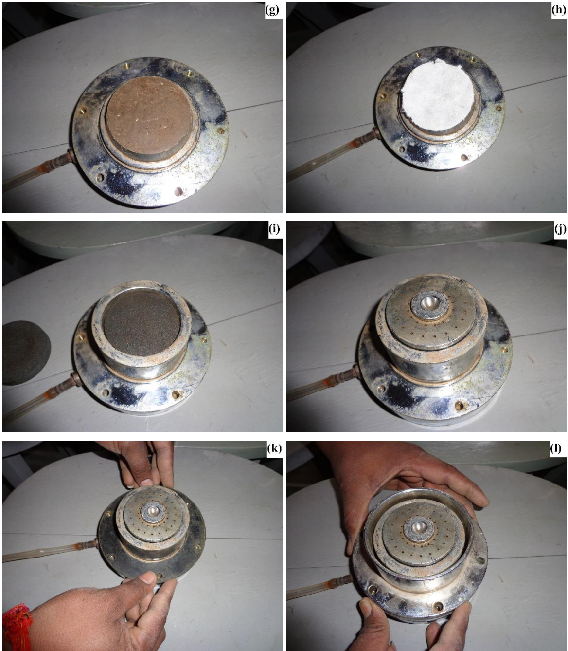
Fig. 3.11 Sequential steps for sample preparation for one dimensional consolidation and swelling pressure testing from: (a) to (l)
