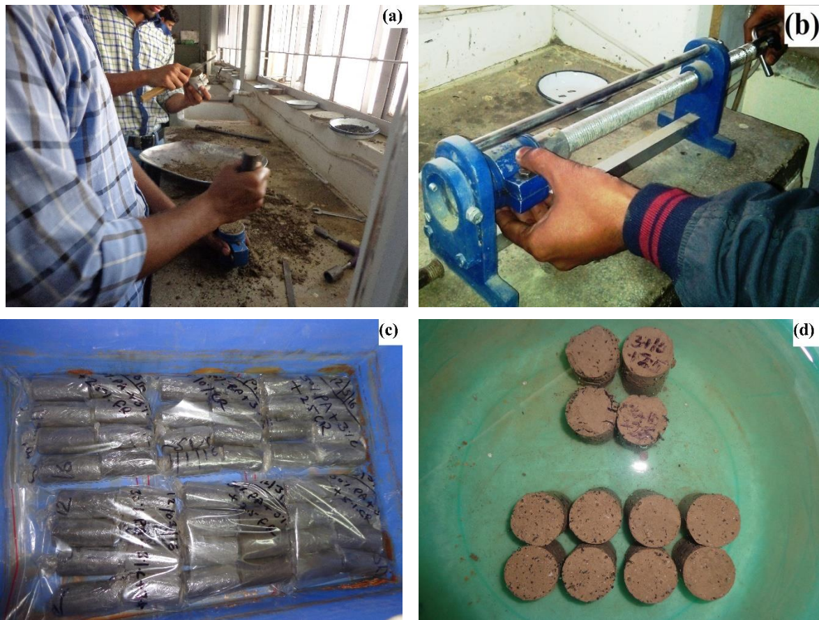
Fig.3.8 Sequential steps for sample preparation for unconfined compressive strength and split tensile strength testing from: (a) to (d)
