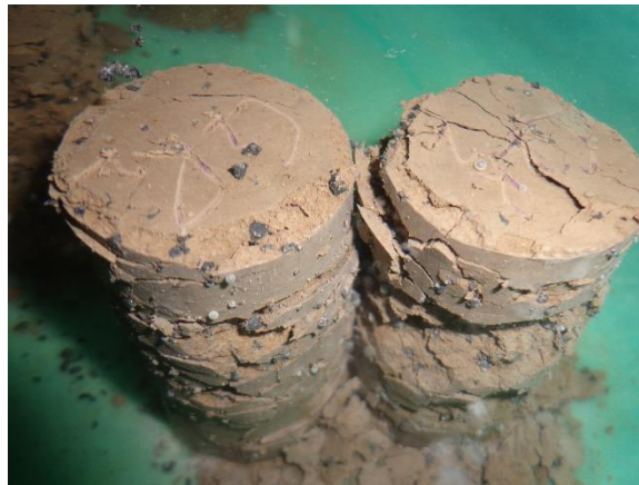
Fig. 5.9 Disintegration of specimens after being immersed in water.
