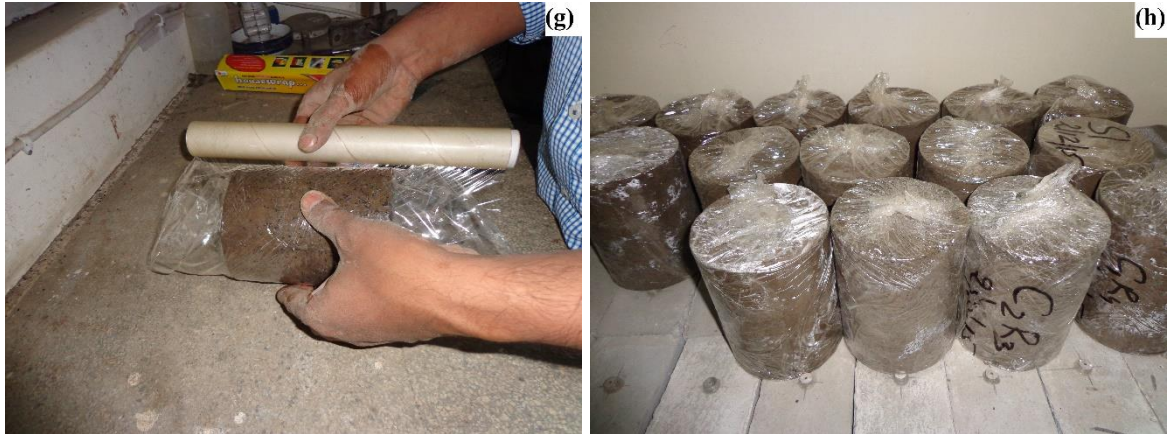
Fig. 3.12 Sequential steps for sample preparation for wet/dry durability testing from: (a) to (h)
