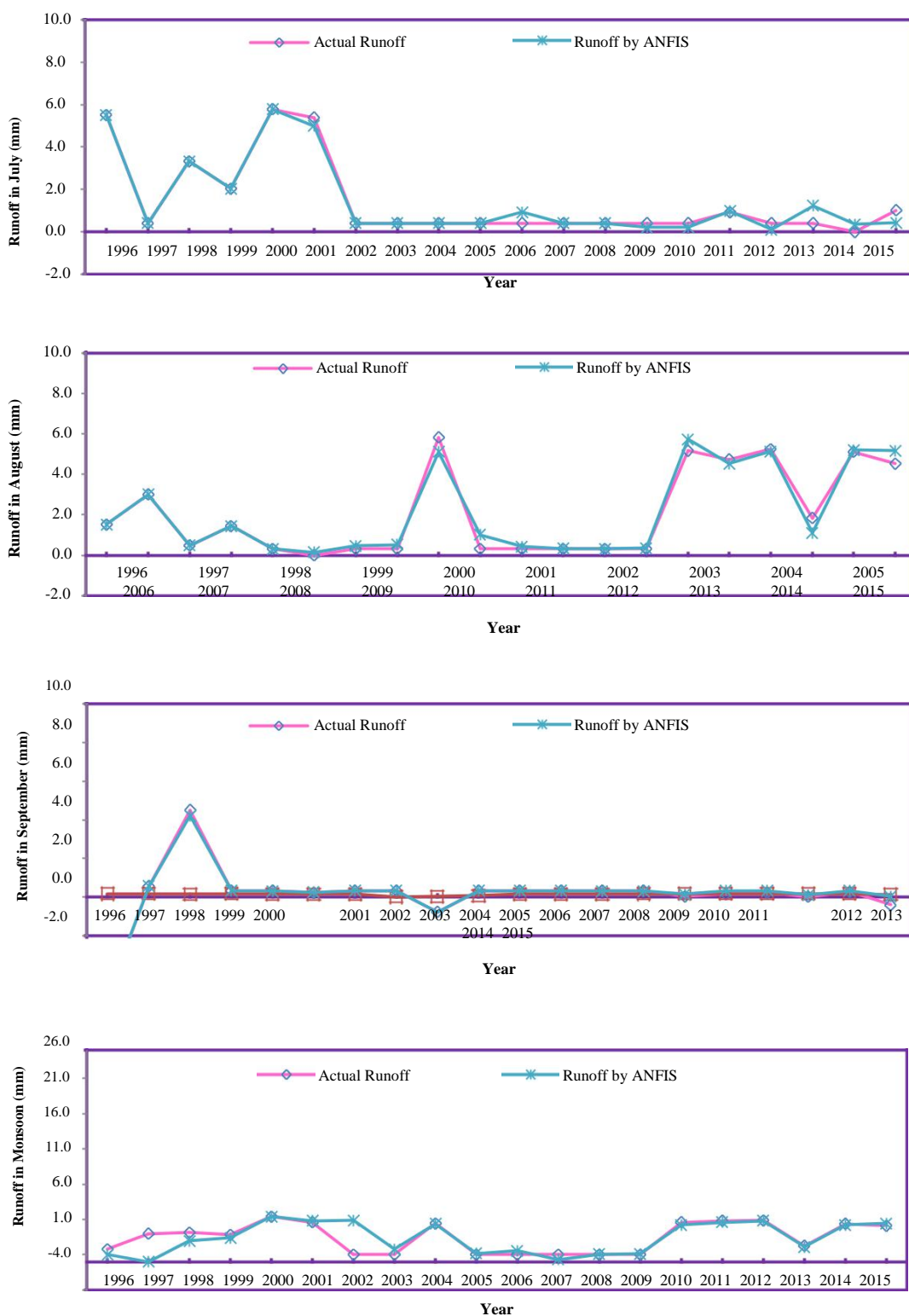
Fig. 5.32: Comparison of actual runoff and runoff predicted by ANFIS model for Lassaria Dam Catchment
