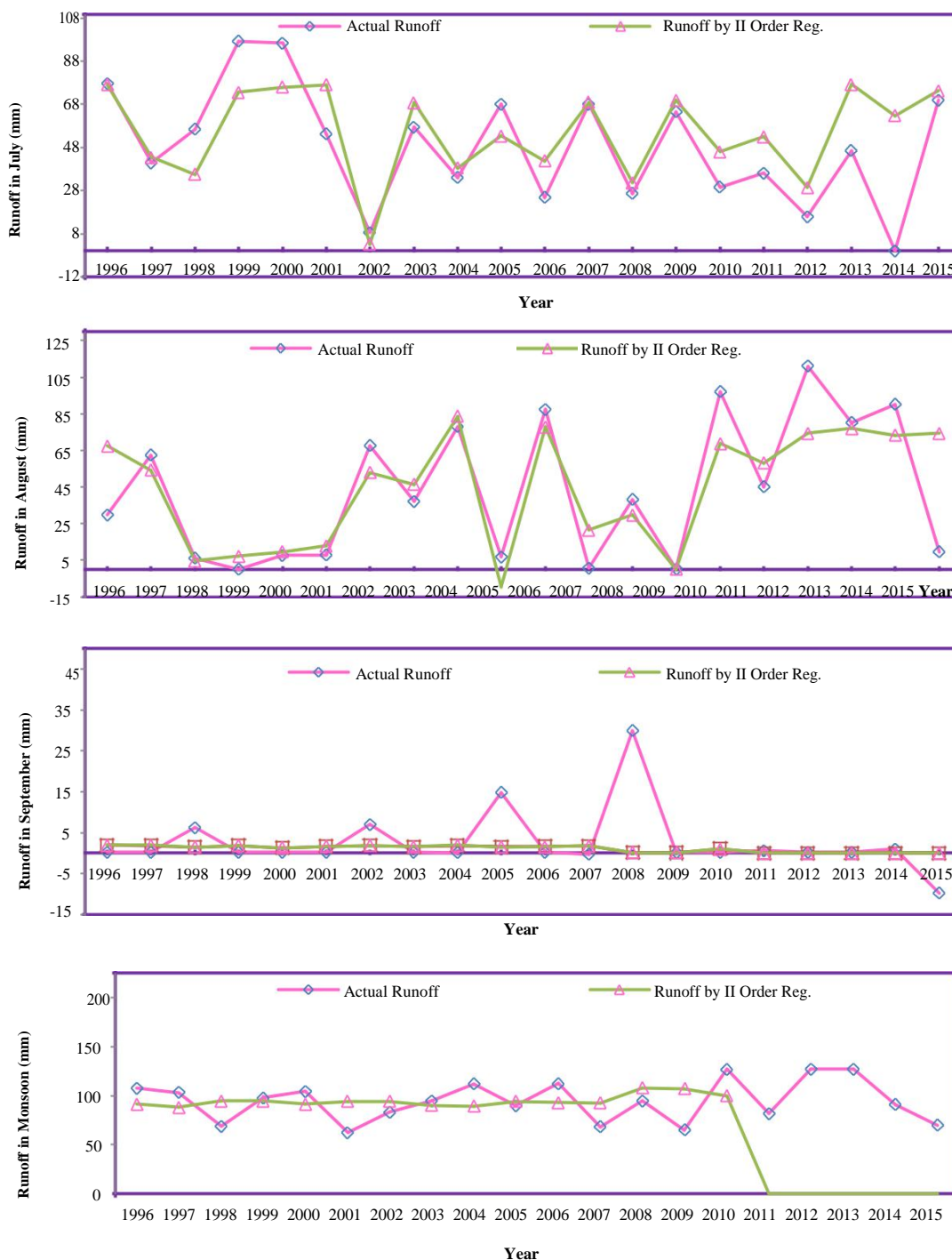
Fig. 5.11: Comparison of actual runoff and runoff predicted by second order regression model for Jetpura Dam Catchment
