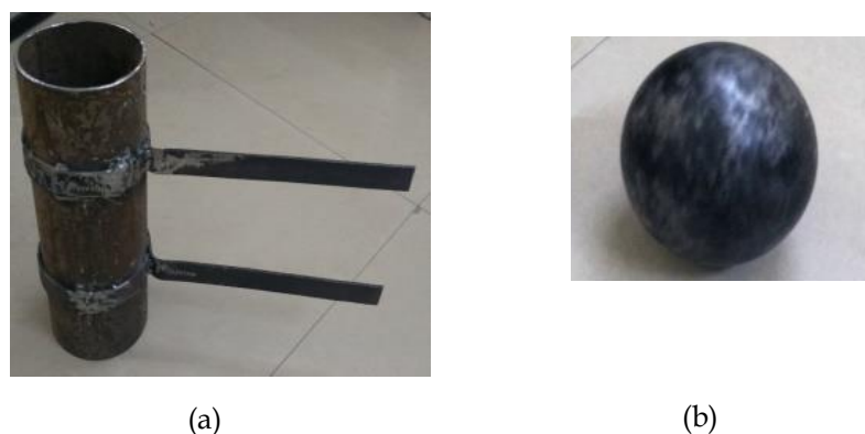
Fig. 3-20: Drop-weight impact test apparatus; (a) guiding assembly and (b) impacter
