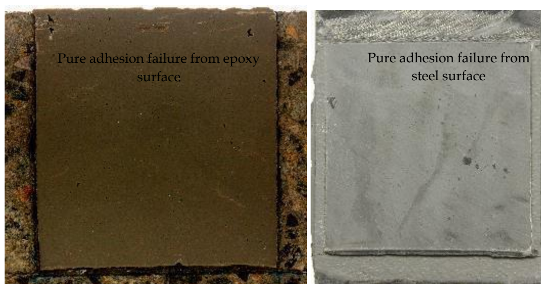
Fig. 6-8: Adhesion failure of one mm thick adhesive layer from epoxy-steel interface
