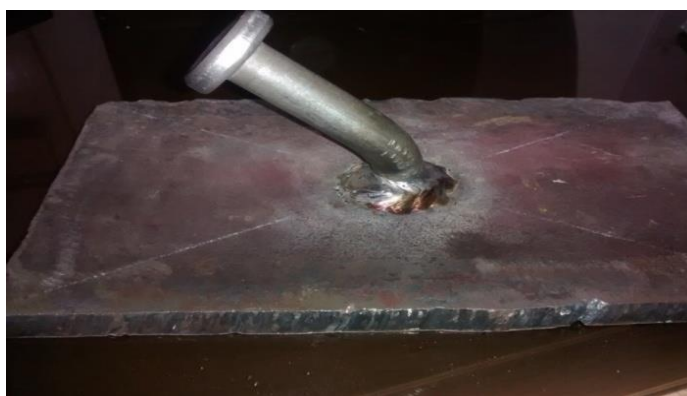
Fig. 3-7: Deformed headed stud connector after bend test
