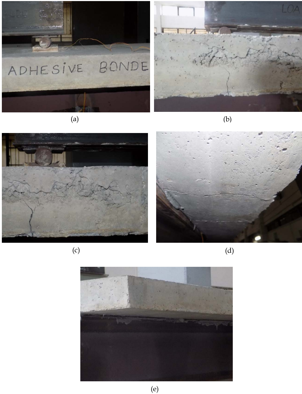
Fig. 7-21: Adhesive bonded steel-concrete composite beam failure; (a) minor cracking in concrete slab below the loaded area (one point), (b) tensile crack opening in concrete slab below the loaded area, (c) increment in crack opening width, (d) through transvers cracking at bottom and (e) bond failure at steel-concrete composite interface
