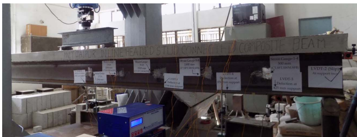
Fig. 7-6: steel-concrete composite beam with the instrumentation arrangement
