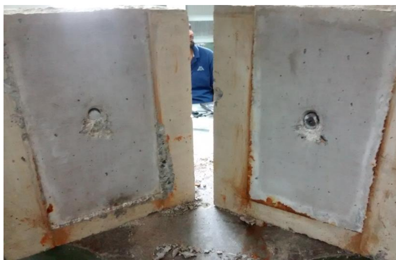
Fig. 5-25: Typical failure of triple layered specimen from both faces (one side stud and other side weld) at the same time
