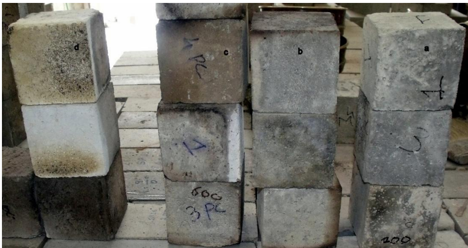
Figure 5.26 Concrete mix C3 after exposed to (a) 200 °C, (b) 400 °C, (c) 600 °C and (d) 800 °C
