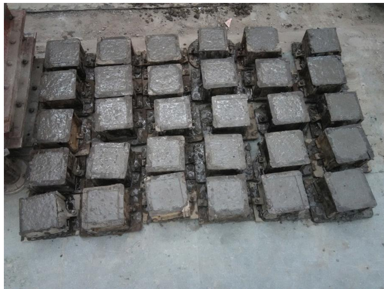
Figure 4.5 Casting of specimens
