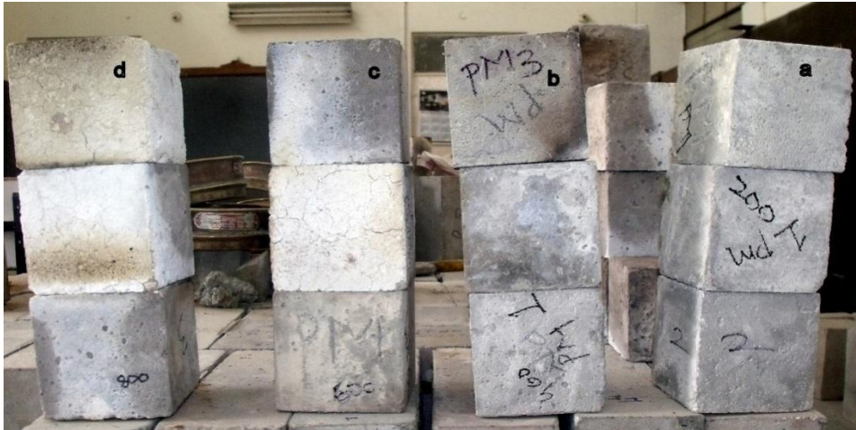
Figure 5.27 Concrete mix C4 after exposed to (a) 200 °C, (b) 400 °C, (c) 600 °C and (d) 800 °C
