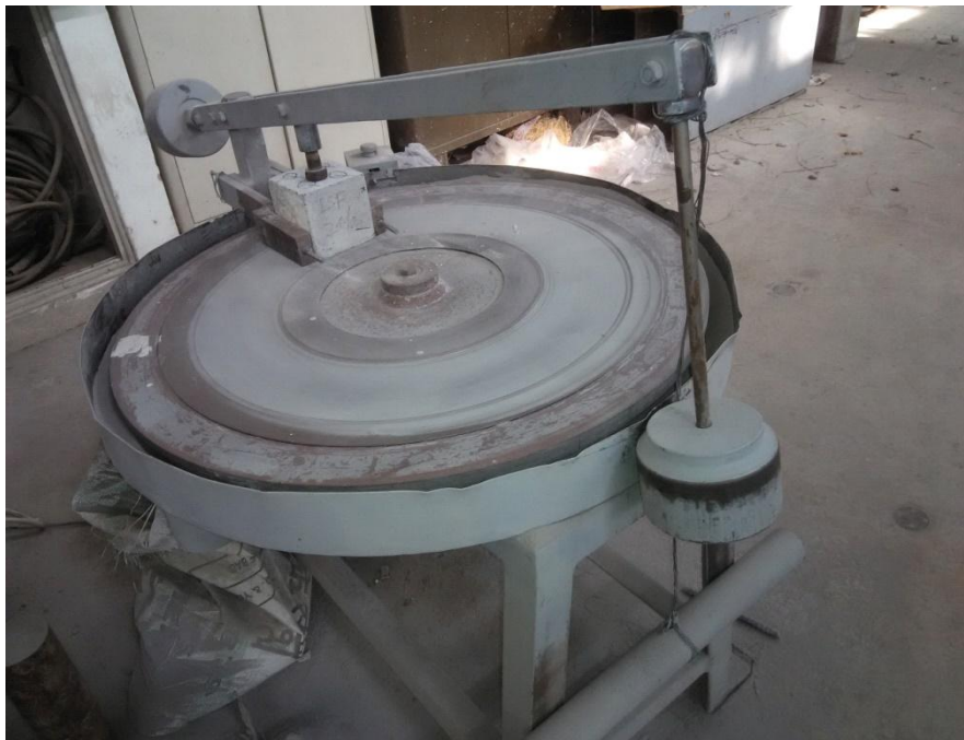
Figure 4.10 Test set up for Abrasion test
