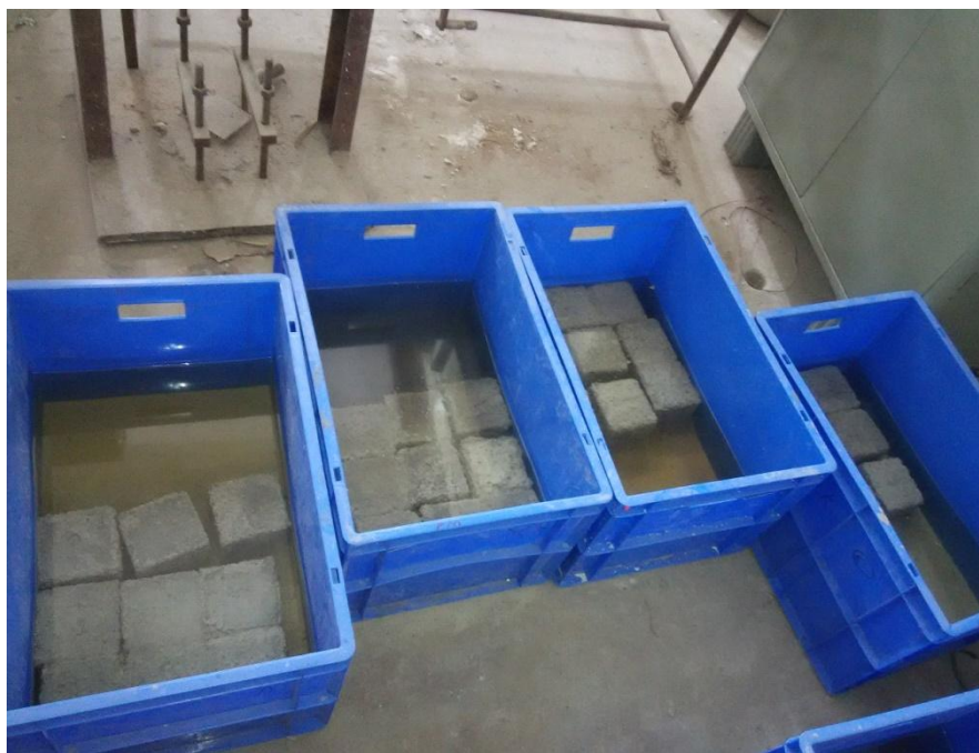
Figure 4.13 Specimens immersed in sulfuric acid solution
