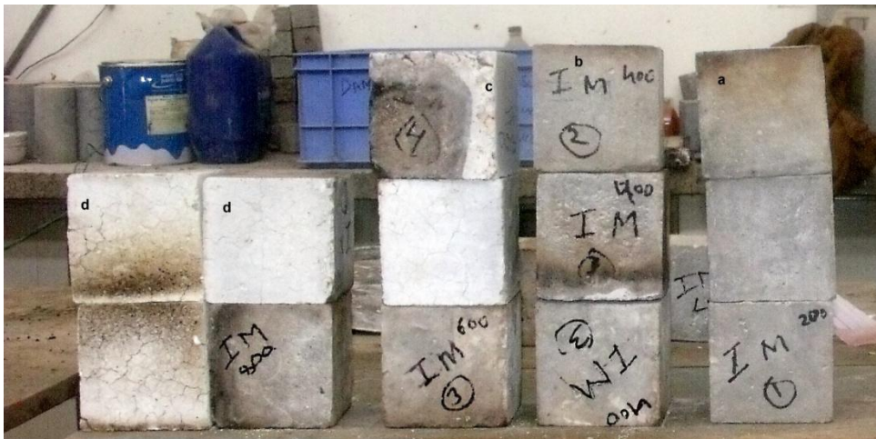
Figure 5.25 Concrete mix C2 after exposed to (a) 200 °C, (b) 400 °C, (c) 600 °C and (d) 800 °C
