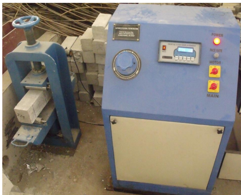
Figure 4.7 Flexural strength test setup
