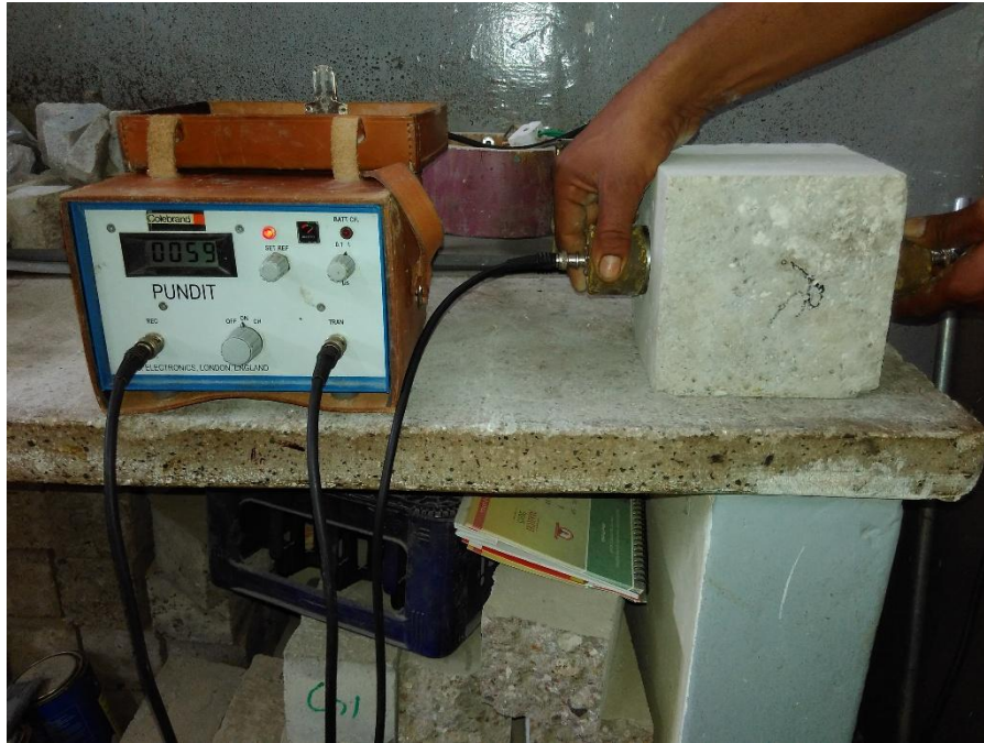
Figure 4.9 Ultra Sonic Pulse Velocity Tests set up
