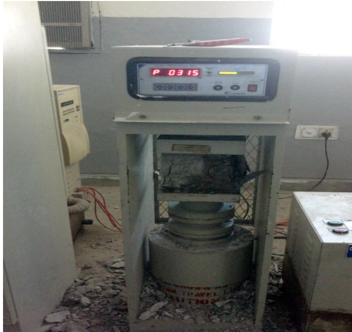
Figure 4.6 Compressive strength test set up
