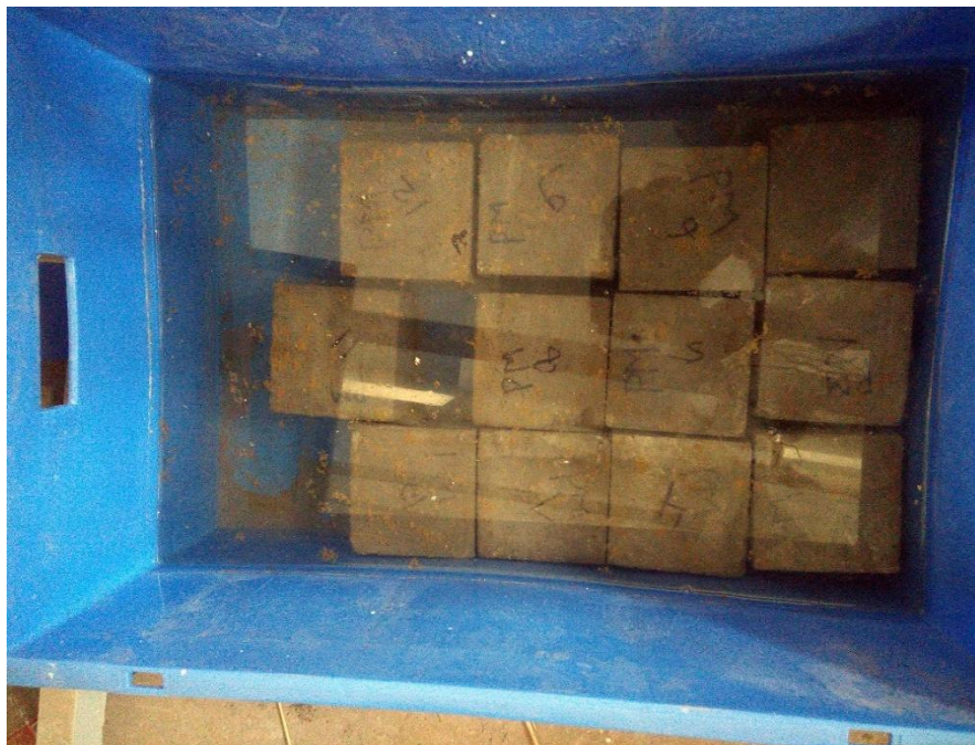
Figure 4.12 Specimens immersed in Magnesium Sulfate solution
