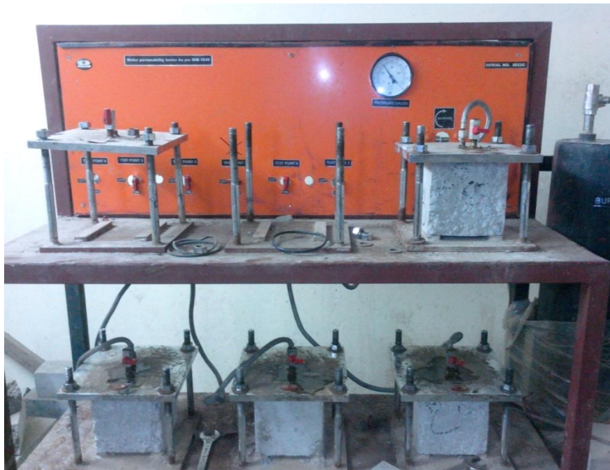
Figure 4.8 Water Permeability test set up
