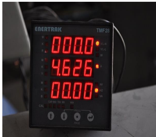
Fig. 3.3.1.7 Digital energy meter used for experimentation
