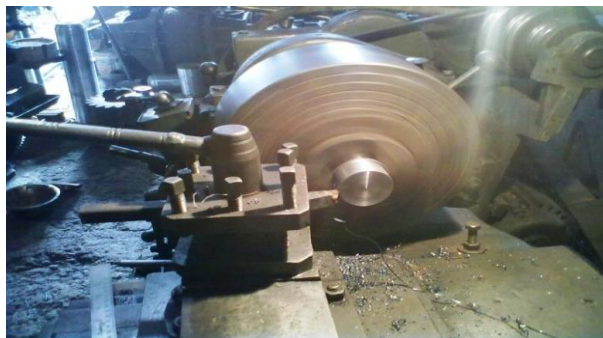
Figure.18 Turning of circular rings on lathe
