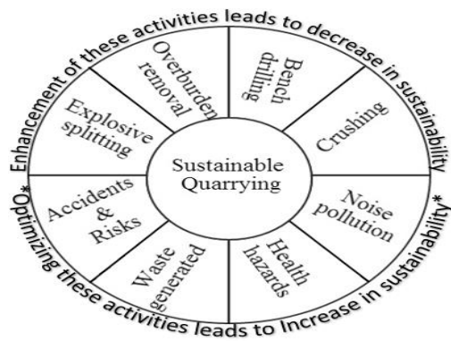
Fig. 4.1.2 Doughnut model for quarrying process
