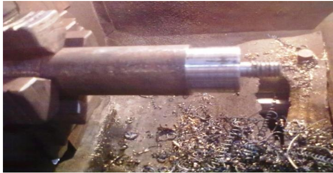
Figure.19 Mandrel for fixing the circular rings on the milling machine
