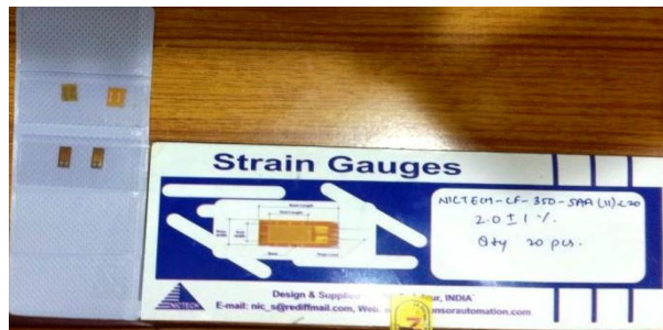
Figure.21 Strain gauges used for dynamometer
