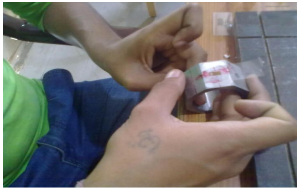
Figure.27 Bonding of strain gauge on the octagonal ring
