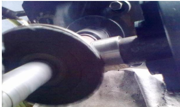
Figure.20 Fabrication of octagonal faces on the outer periphery of rings.
