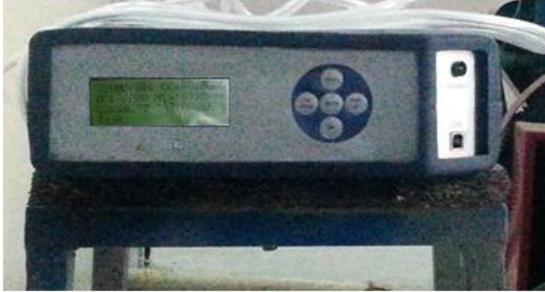
**Fig: 3.4 AVL Exhaust gas analyzer**
