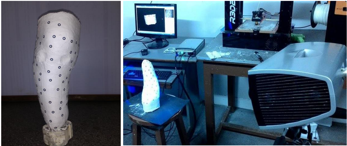
Figure 5.1 The Plaster of Paris socket model (left), 3D scanning arrangement (right)
