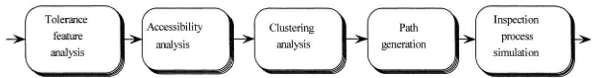
Figure 2.14 The inspection path planning for CMM (Zhang et al. 2000)
