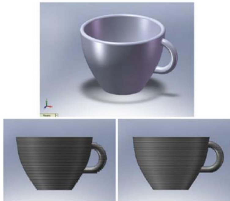
Figure 2.1 Layer variation in AM process (Gibson et al., 2014)
