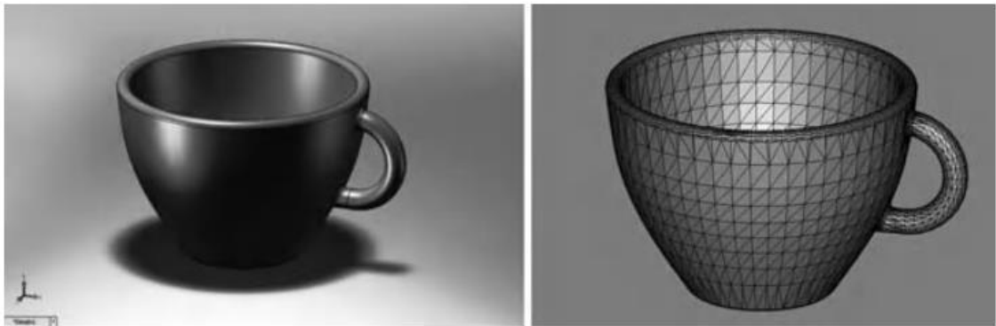
Figure 2.5 Conversion of CAD model (left) into STL model (right) for FDM fabrication (Gibson et al., 2010)
