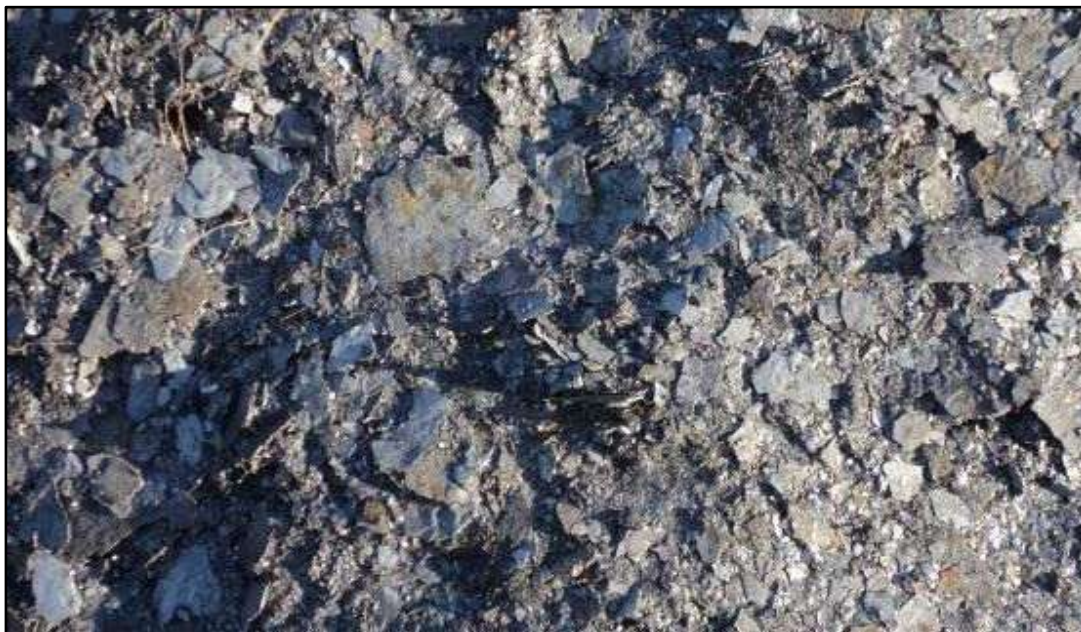
Figure-2.10: Mill scale wastage produced during hot rolling
