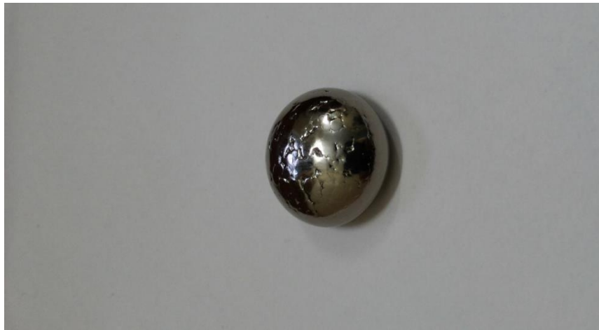
Figure 3.2: Ingot of bulk amorphous Zr_{55}Cu_{30}Ni_5Al_{10} alloy
