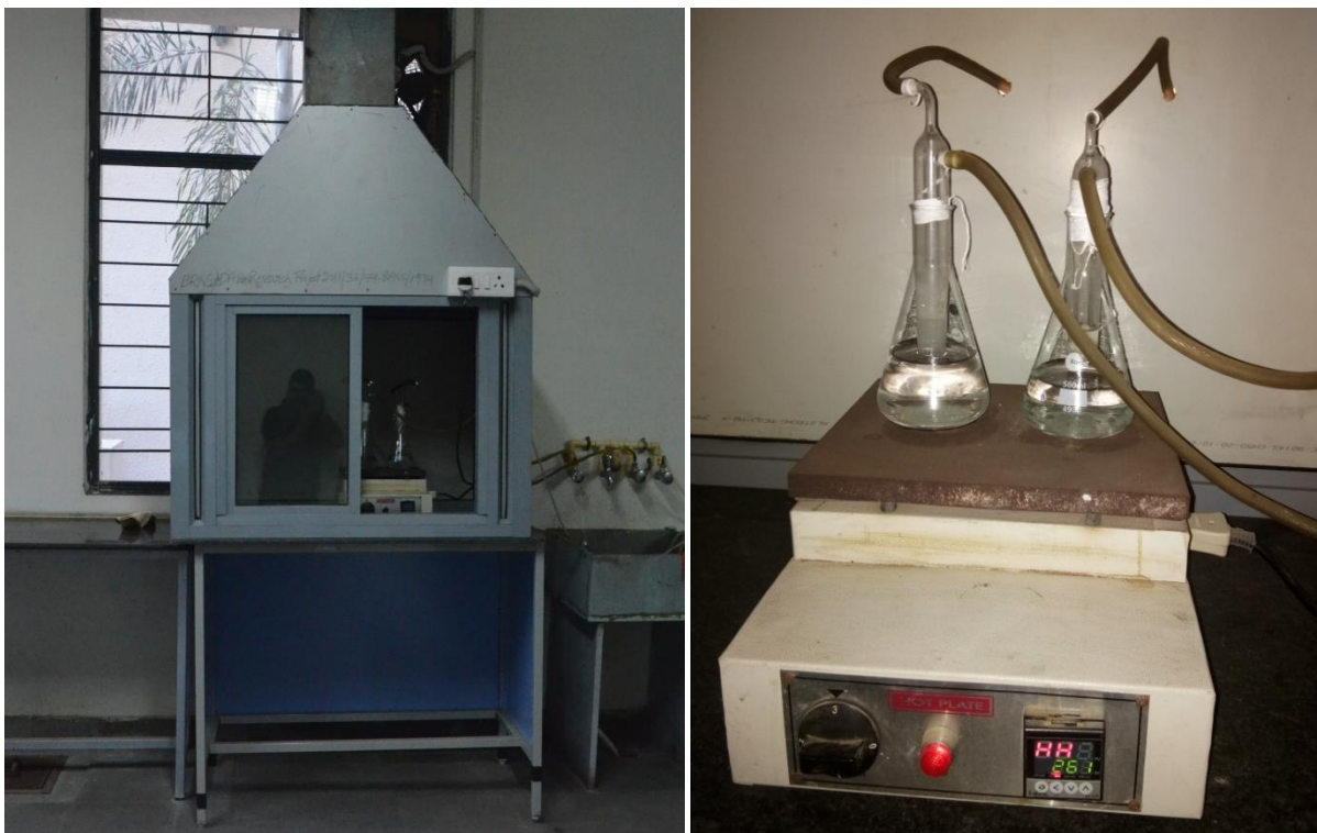
Figure 3.8: The experimental setup for high temperature corrosion studies
