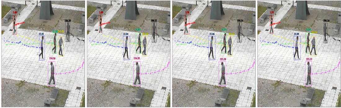
Figure 5.11: Frame sequence from synopsis video assigned a time stamp to each object. Here, time stamp is used as indexing of object in original video.
