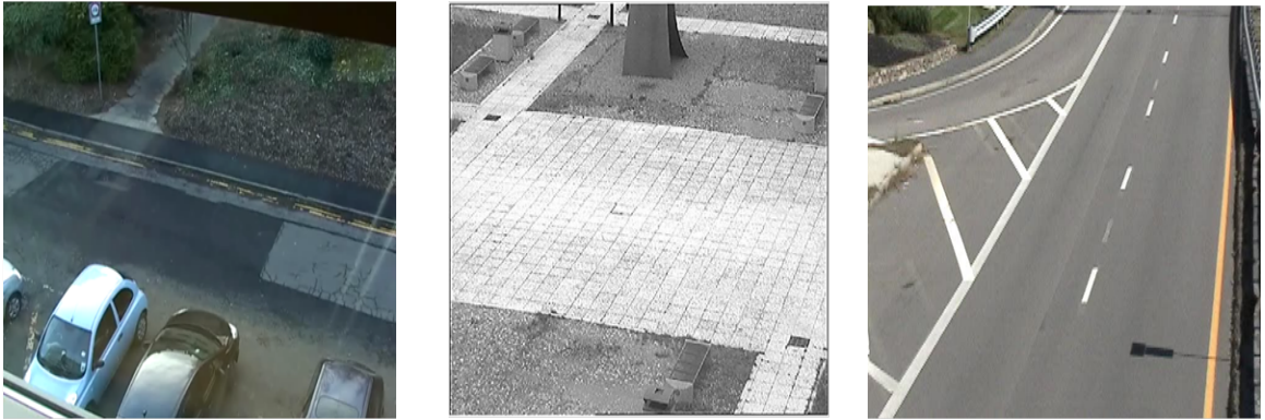
Figure 5.3: Background images of three different videos used in generating synopsis video. Initial image sequence without any moving object is selected as a background image for temporal shift of object from original video.
