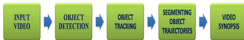
Figure 1.2: System overview of generating synopsis video in this work. Given a set of video frames, the task is to generate the synopsis video of important activities.
