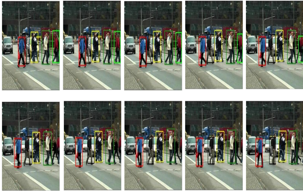
Figure 4.8: Qualitative analysis of tracking using proposed method over TUD – Crossing video of PETS2009 dataset from frame 89 to frame 98. Occluded objects are tracked successfully using proposed approach.
